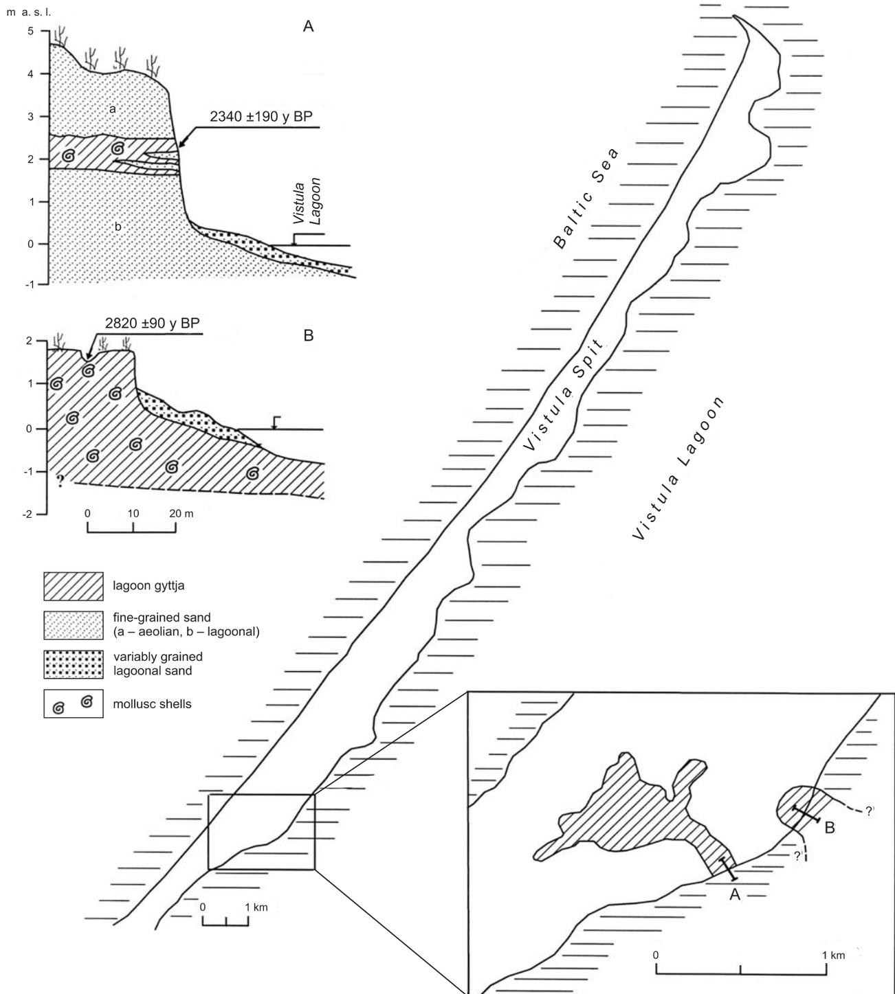
**Fig. 2.** Location of lagoon gytija in the central part of the Vistula Spit (enlarged area) and geological settings of the investigated sections (geological cross-sections along lines A and B)
