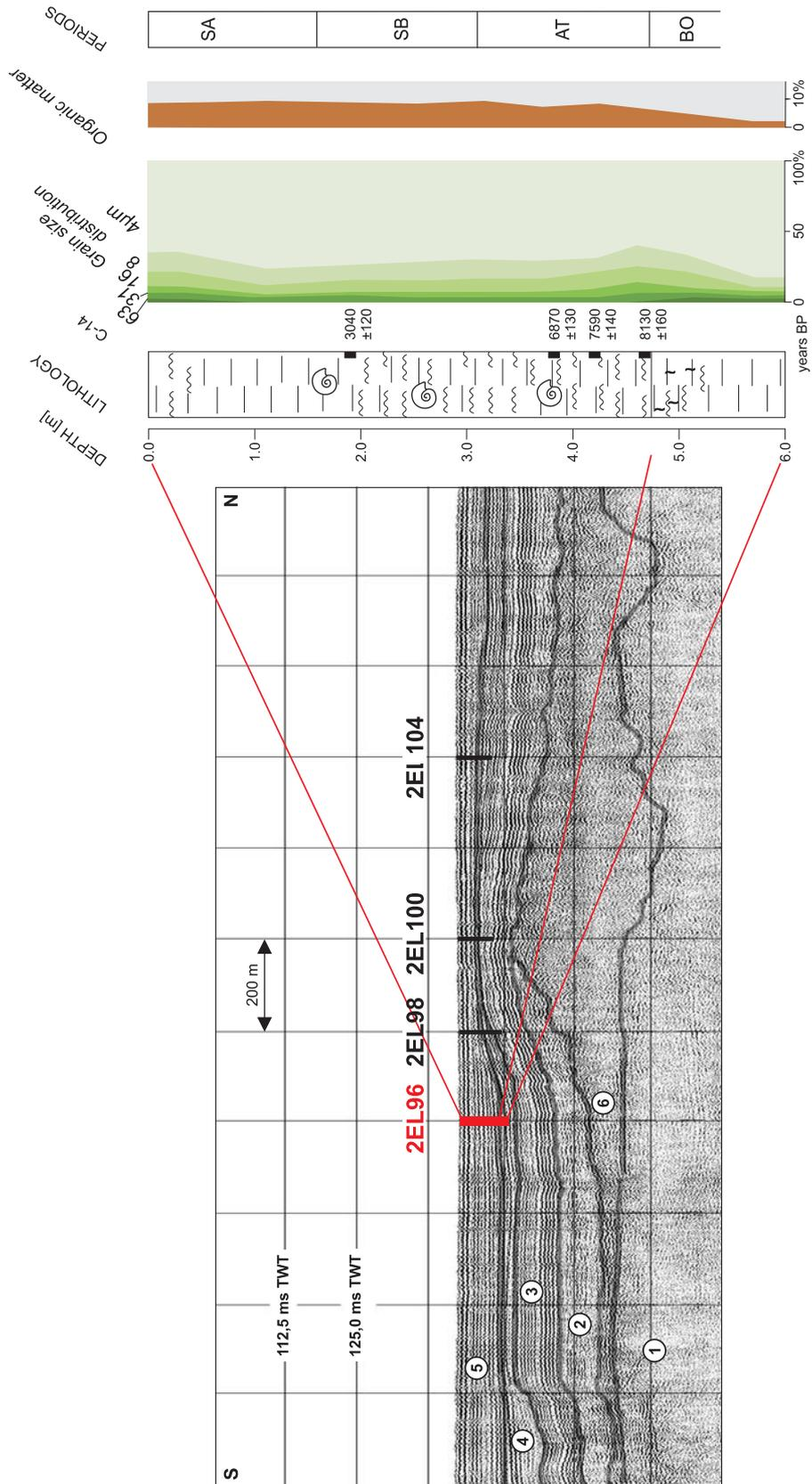
Fig. 15. The seismoacoustic profile of the Gdansk Basin across 2EL/96 coring site
