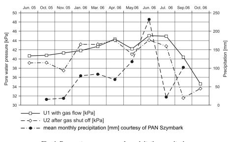
Fig. 4. Pore water pressures and precipitation monitoring
