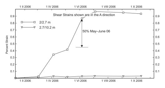
Fig. 3. Interpretation of mass movements measurements, displacement/shear strain plots
