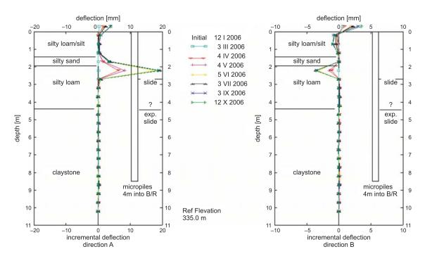
Fig. 2. Results of ground movement measurements
