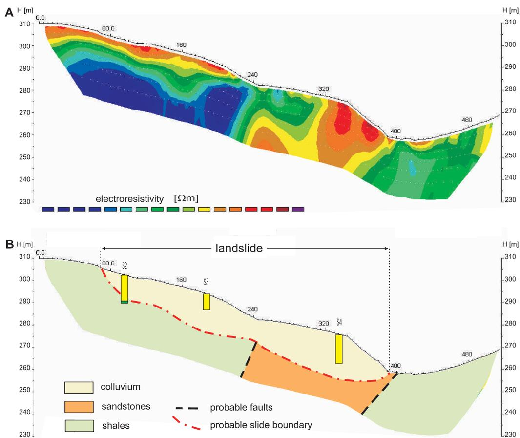
Fig. 5. Geophysical results of Dubiecko landslide investigations
