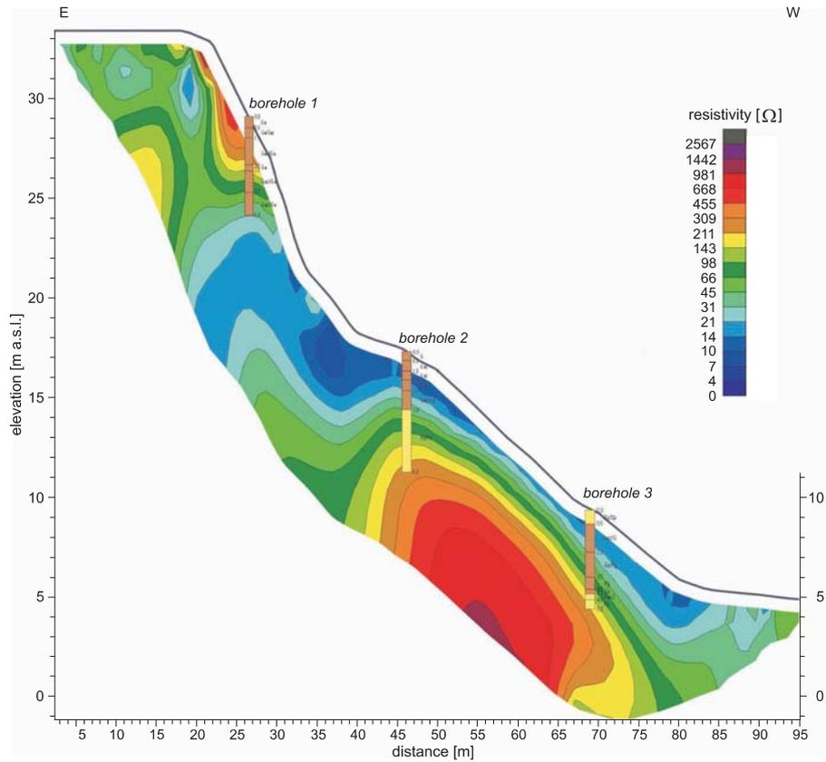
Fig. 9. Resistivity cross-section on the basis of Electric Resistivity Tomography profile, landslide Malbork
