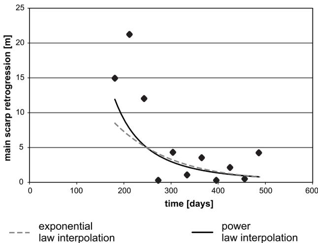
Fig. 11. Main scarp retrogression during June 1995–May 1996
