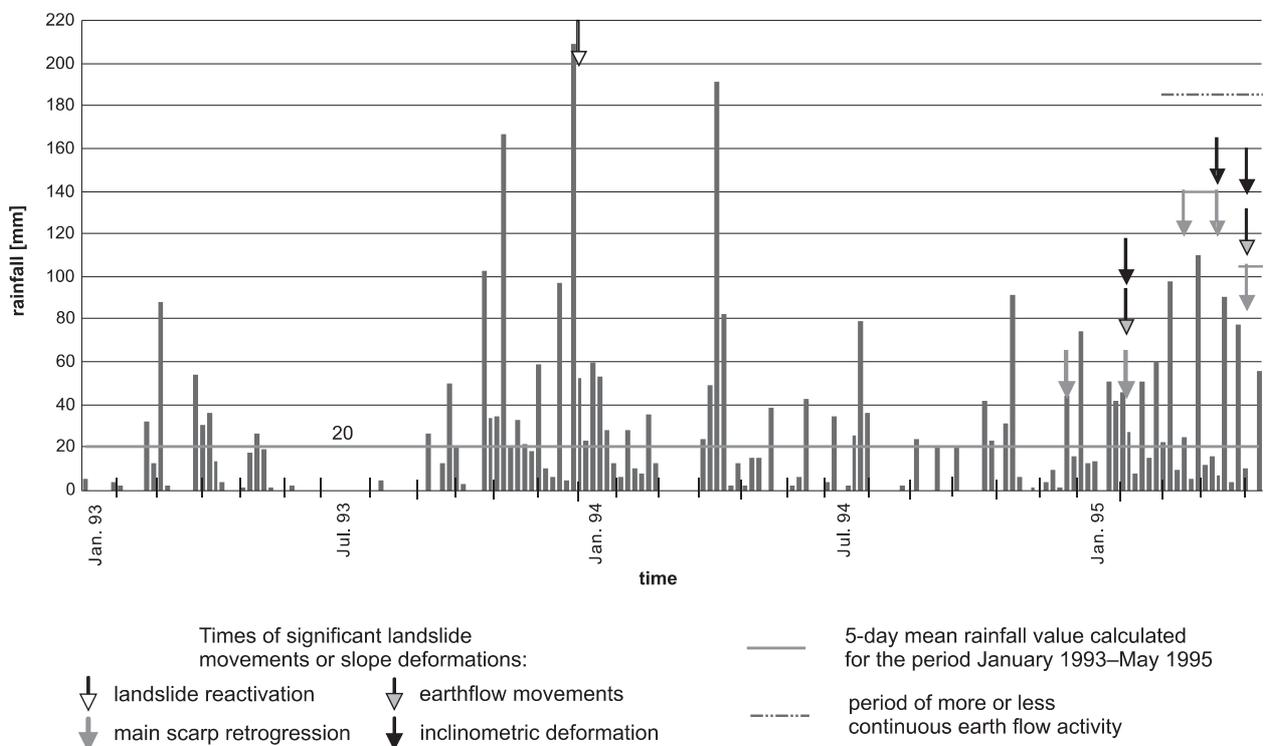
**Fig. 5. Five-day cumulative rainfall at the Senerchia rain gauge and landslide activity**
