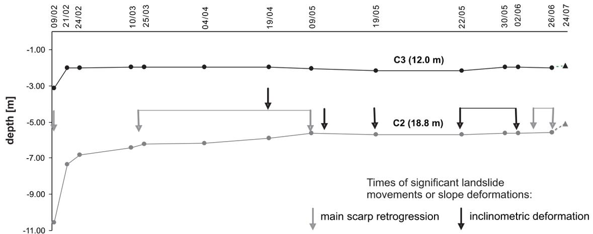
Fig. 7. Variation of piezometric levels in borehole P4 sited in the crown — main scarp area and landslide activity between February and July 1995
