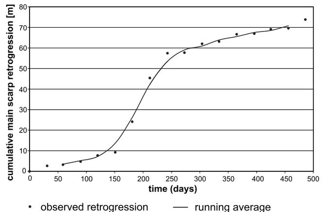
Fig. 12. Main scarp cumulative retrogression during the June 1995–May 1996 period, and moving average (continuous line) calculated on the three successive measurements
