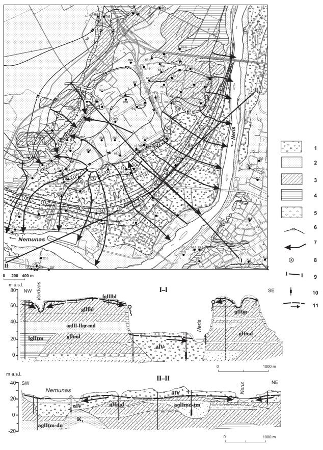
Fig. 1. Hydrodynamic scheme of shallow groundwater outflow estimation in contact of alluvium and fluvioglacial sediments
