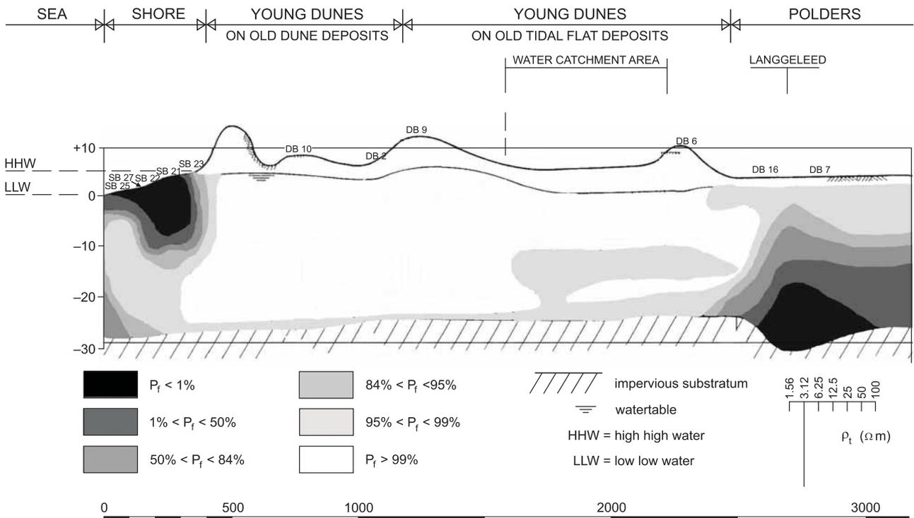
**Fig. 2. Cross-section through the shore, dunes with the water catchment and polder**
