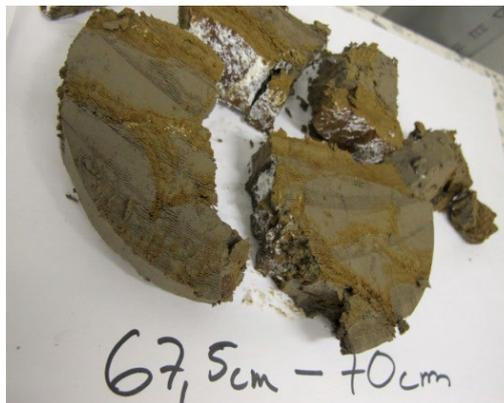
Fig. 3 (on the right). Cross-section of a soil sample after the flow of 6.4 dm<sup>3</sup> of calcium carbonate suspension through the column during eight days.
