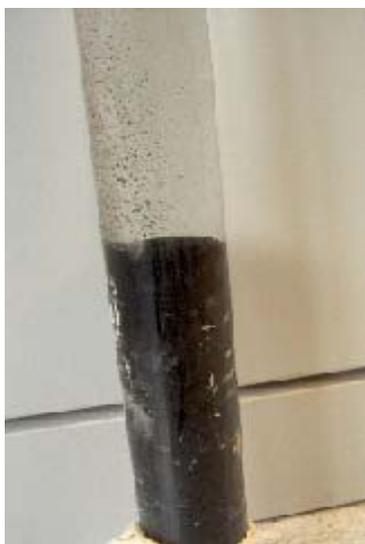
**Figure 3.2. Photo of the sediment core in plastic pipe**
