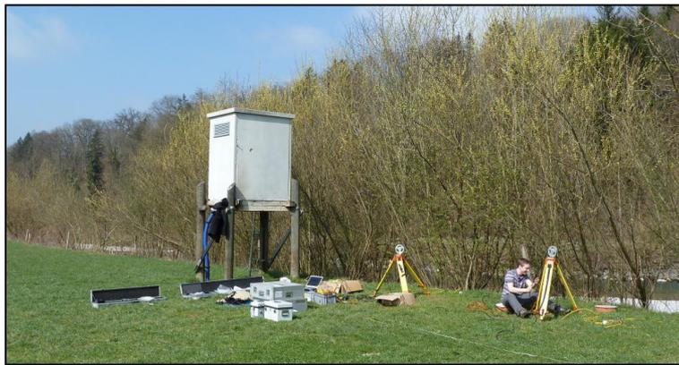
**Figure 1.3.** Crosshole GPR acquisition at the Widen field site.
