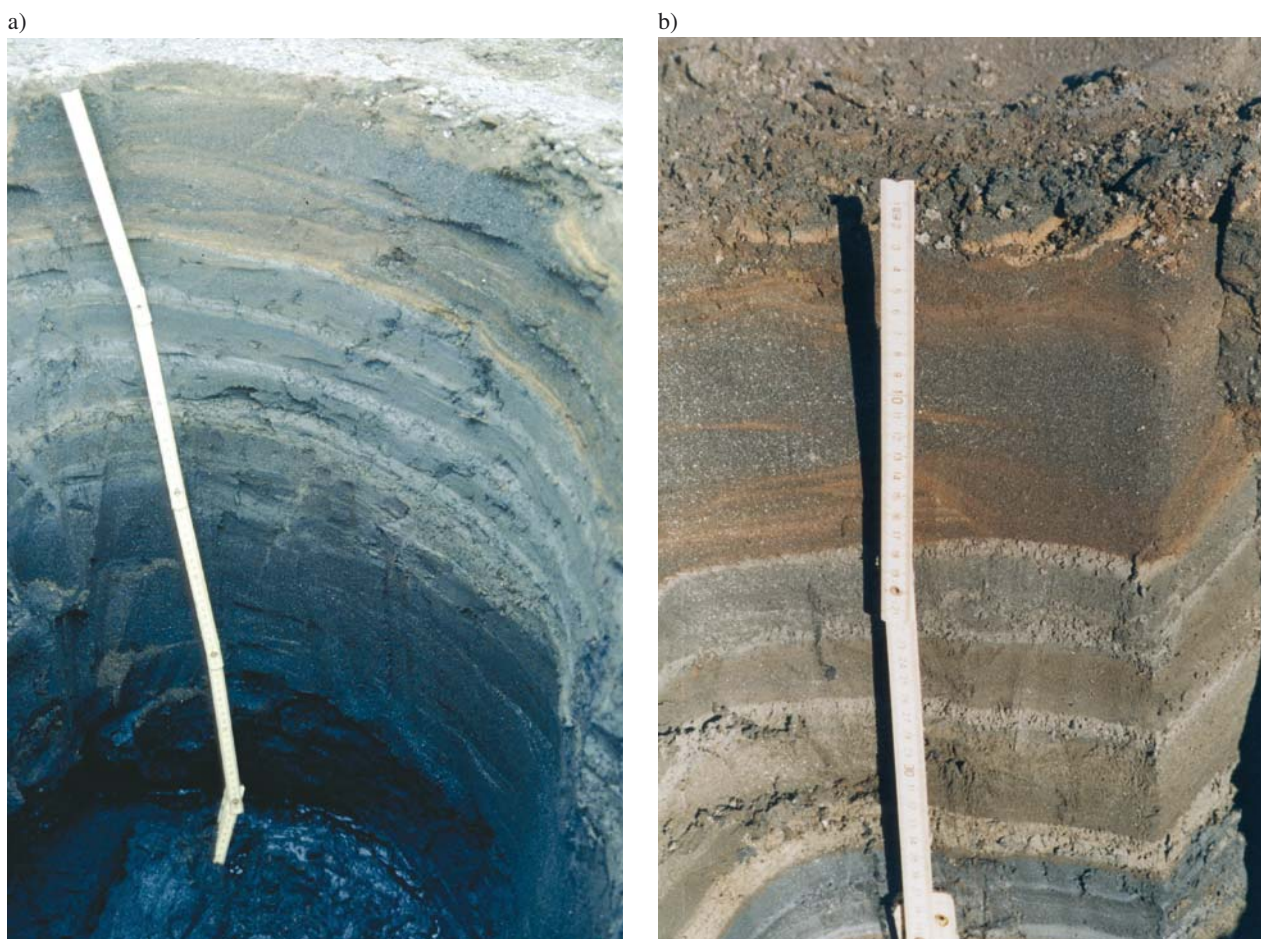
Figure 27. The present-state environmental assessment includes investigation of chemical weathering of mineral grains in tailings deposits, in order to evaluate the need for covering procedures. Tailings samples are collected for analysis from excavated test pits (as shown here) or by drilling profiles through the tailings into the underlying substrate. Tailings deposits exposed here show the effects of oxidation of sulphides, especially within the uppermost 20 cm of the profile.
