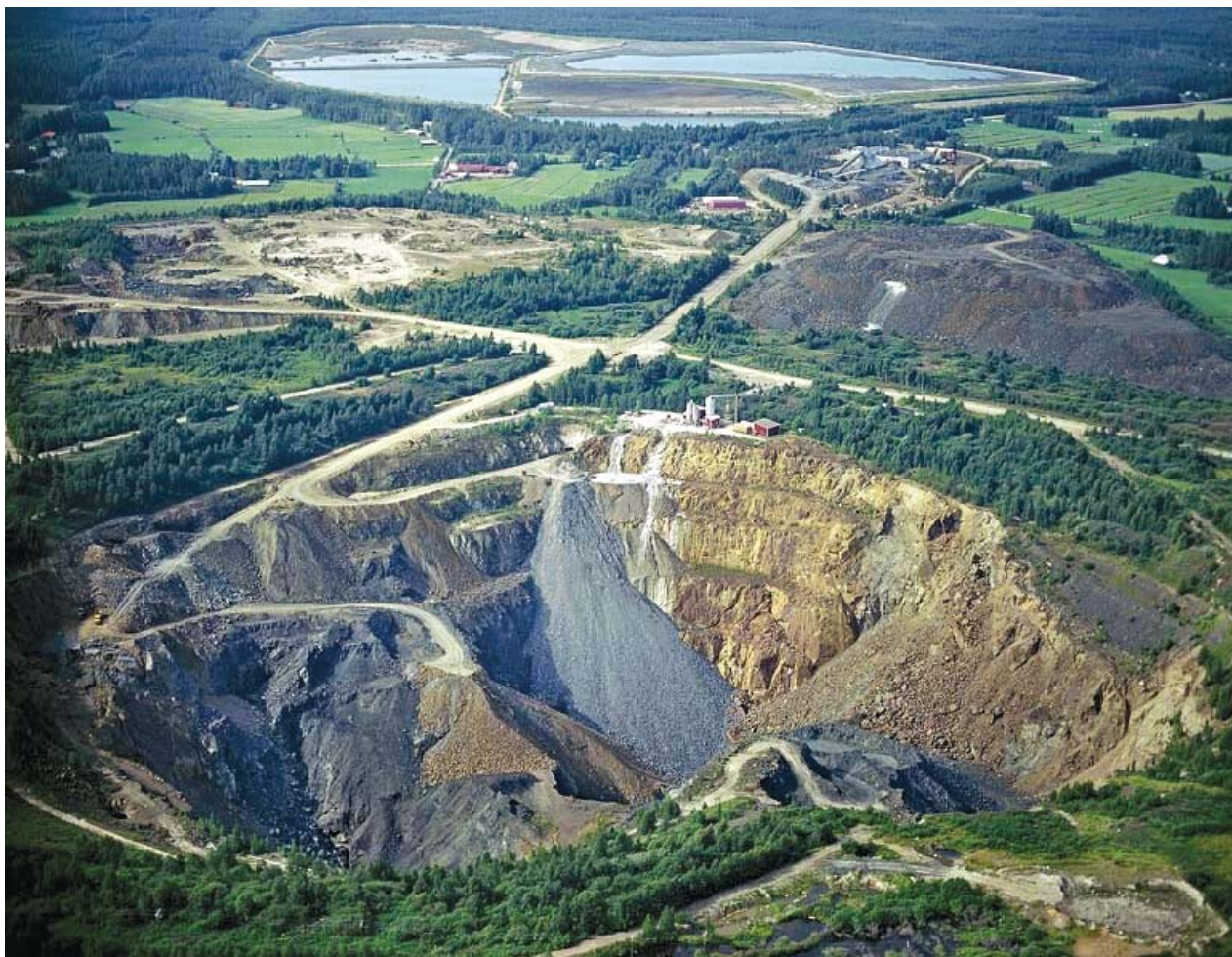
Figure 1. Hitura Ni-Cu mine, Nivala, Finland. Open pit is in the foreground, with waste rock and overburden stockpiles and concentrator plant behind. Tailings impoundment and settling ponds are visible in the background.
