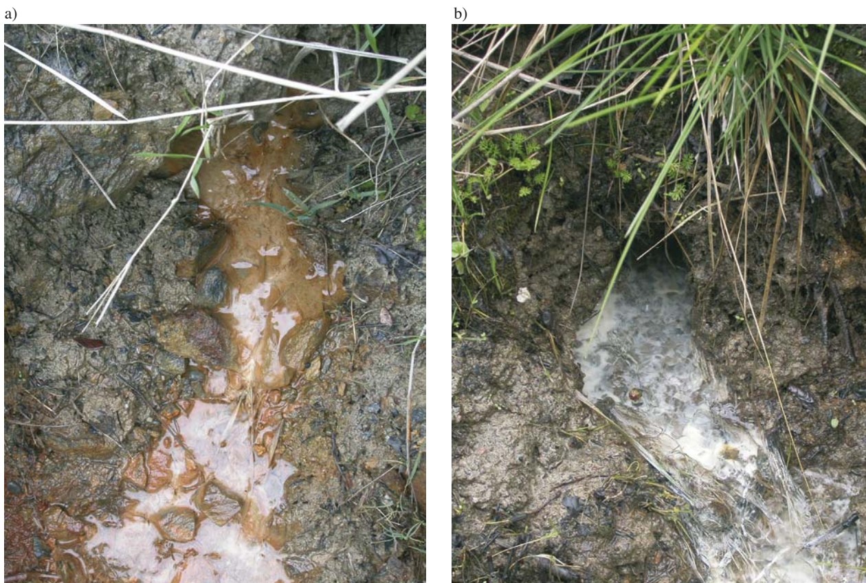
Figure 23. Surveys of the distribution and composition of seepage water are aimed at documenting current and potential discharge sites from tailings and waste rock areas to assist in closure planning and ongoing site monitoring. Seepage water discharge under acidic conditions can precipitate iron-, aluminium and/or manganese hydroxides or oxyhydroxides on grain surfaces, which are discernible as reddish (a), yellowish or whitish (b) coatings and aggregates.
