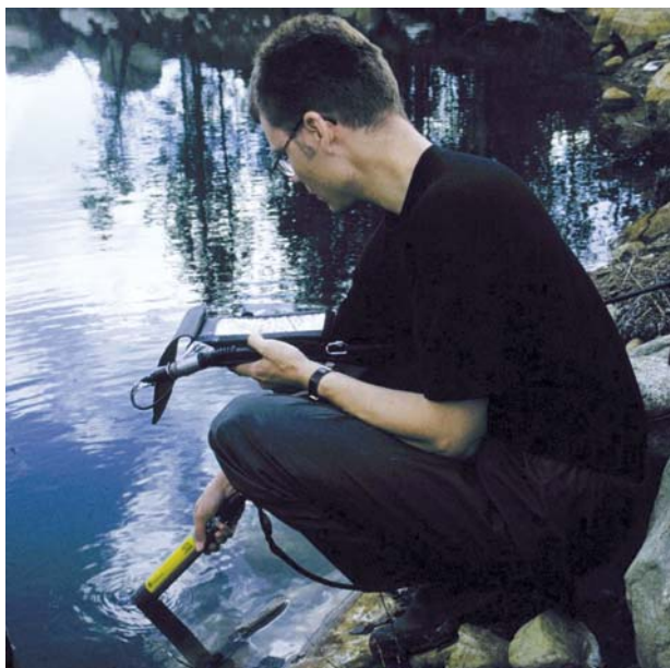
Figure 49. Following mine closure, monitoring of surface and groundwater quality involves in situ measurement of certain parameters, such as pH, electrical conductivity and oxygen, in addition to laboratory analyses.
