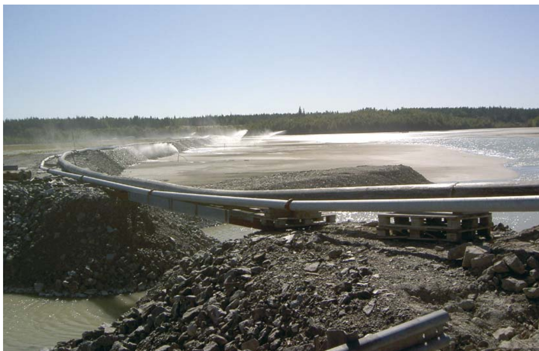
Figure 6. Generation of dust from tailings areas can be minimized by watering (as in picture) or spreading a lime slurry (Zinkgruvan Zn-Pb mine, Sweden).
