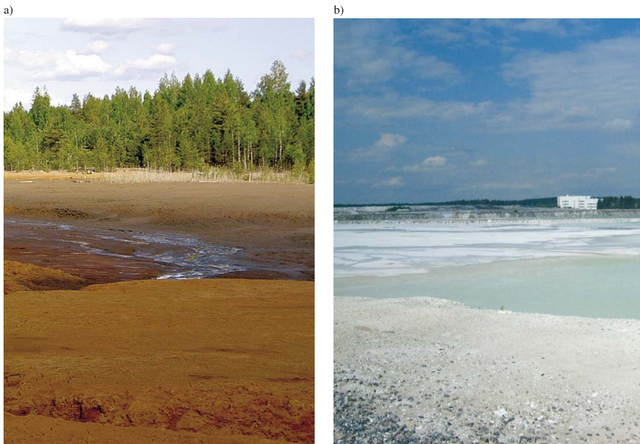
Figure 39. Mineralogical and chemical composition of tailings exerts a strong influence on long-term behaviour. a) Sulphide-bearing tailings exposed to the atmosphere are susceptible to oxidation, which may generate acidic, metal-rich runoff and seepage. b) Tailings at carbonate mines tend to be more chemically non-reactive.
