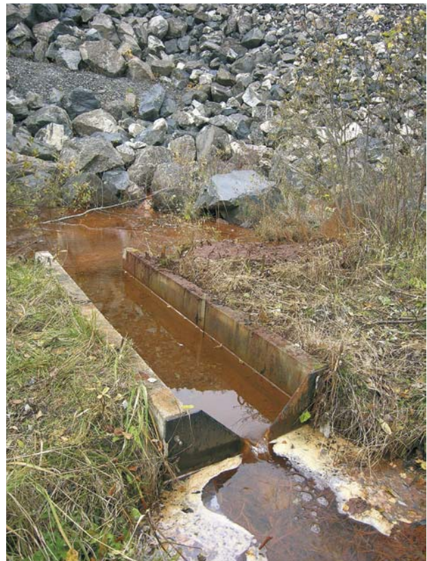
Figure 50. Seepage water discharge rates from waste rock areas and tailings impoundments can be monitored effectively by installation of standard V-shaped water gauges (Vee-weir) at outflow locations.
