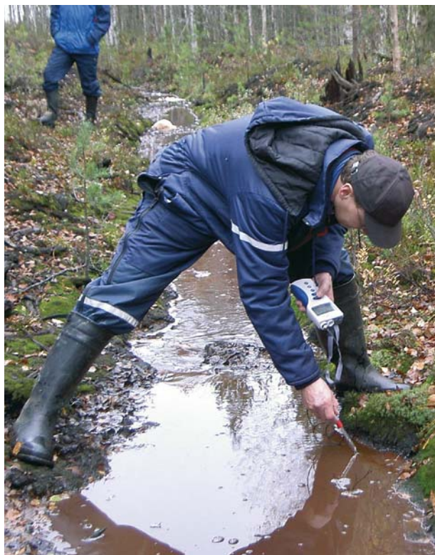
Figure 16. An environmental permit can require the operator to monitor the impact of operations even after operations are discontinued. The monitoring programme may include monitoring of the quality of water discharged from disposal areas. The photo shows Redox measurement of water from a mine site.
