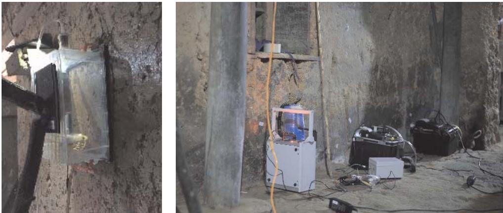
Fig. 2. *Left:* Measurement chamber with optional internal fan is pressed against wall to seal a defined volume of air in contact with a standardized surface area of mud; air is recirculated at  $1 \text{ L min}^{-1}$  through instruments. *Right:* SARAD<sup>®</sup> RTM2200 and two RAD7 units measuring radon and thoron during daytime in the room air of a northern Vietnamese mud house
