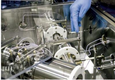
View of the opened source chamber of the SHRIMP IIe/MC, with the primary column and Köhler apertures (location showing by hand) and secondary column extending (to the left) towards the electrostatic analyser
