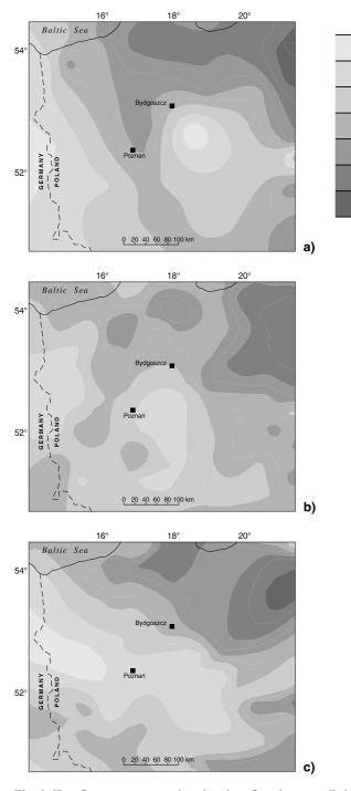
Fig. 2. Heat flow contour maps based on heat flow data compiled by: (a) Plewa (1994), (b) Gordienko and Zavgorodnaya (1996) and (c) Bruszewska (2001). Heat flow contours are in  $mW/m^2$ .
