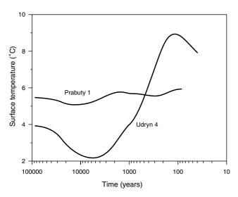
Fig. 5. Ground surface temperature history derived from FSI of the temperature profiles in well Udryń-4 and Prabuty-1. Note that the sharp change observed in Udryń-4 well is not observed in Prabuty-1 well.
