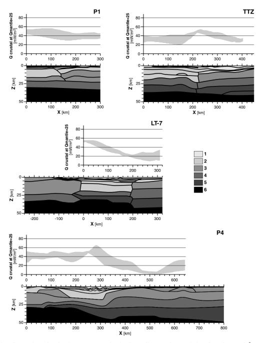
Fig. 7. Crustal heat flow at the surface for the LT-7, TTL and Polonaise profiles assuming mantle heat flow of 25 mW/m<sup>2</sup>. Composition of the individual structural elements of the crust are from Krysiński et al. (2000): 1–sediments, 2–compacted sediments, 3–granitoids, 4–"basaltic" layer, 5–gabbroes, 6–subcrustal mantle (peridotites).
