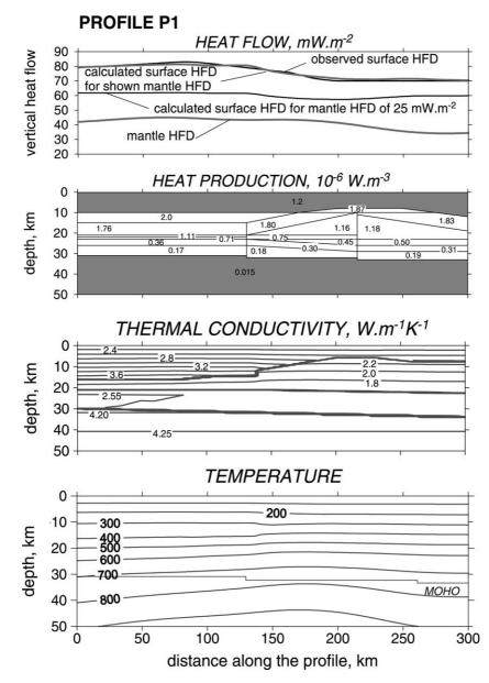
Fig. 8. 2D models of surface and optimised mantle heat flow densities, heat production ( $\mu W m^{-3}$ ), temperature corrected thermal conductivity ( $W m^{-1} K^{-1}$ ) and crustal temperature (°C) for the profile P1.
