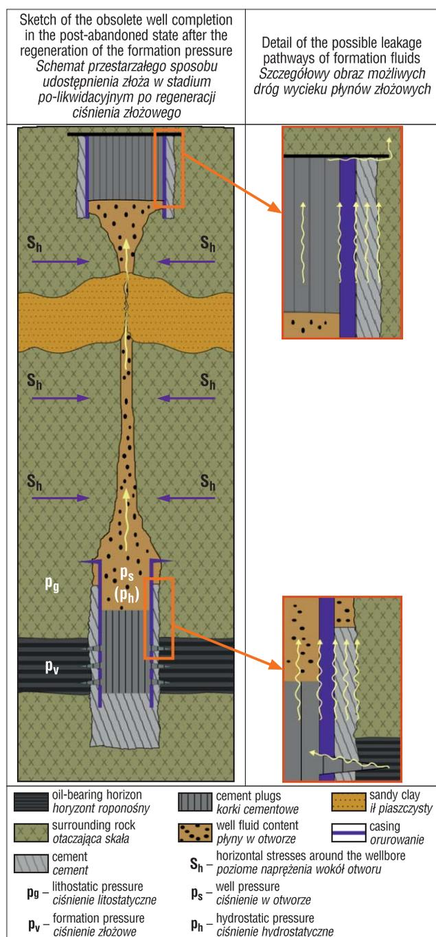
Fig. 9. The scheme of wellbore condition before the definitive re-abandonment procedure (Bujok et al., 2015)
