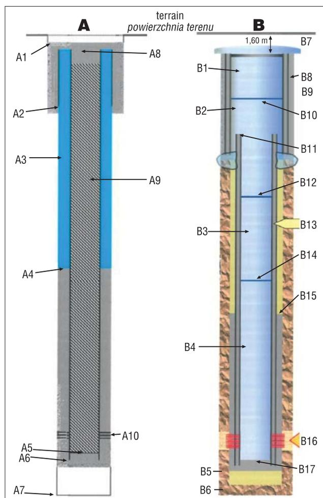
**Fig. 8.** Well H 289. **A** – situation after abandonment in 1965; **B** – situation after re-liquidation in 2014
