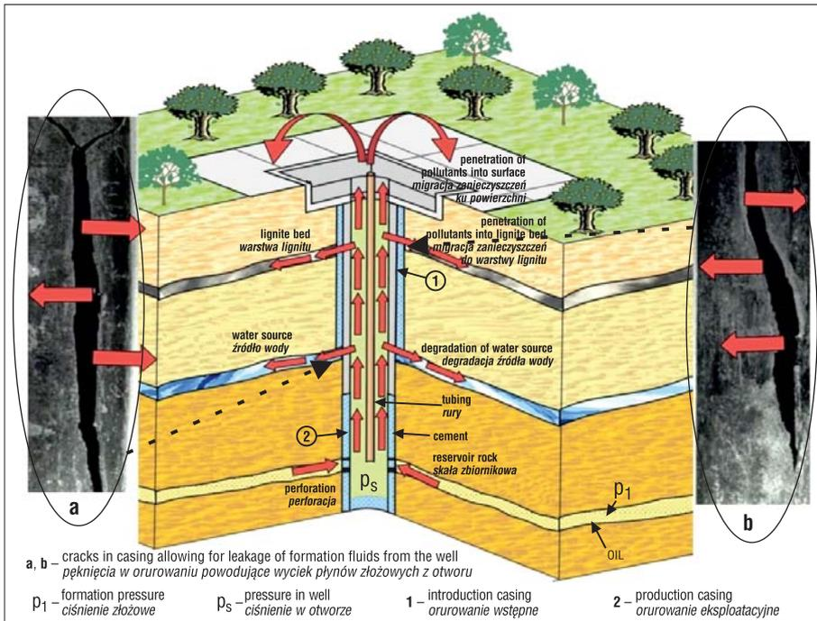
**Fig. 5.** Possible ways of contamination spread through an old, un-abandoned well. Lignite bed is presented on purpose. Intensive mining of lignite took place in the described area in the past (Propagační materiál PKÚ, 2014)
