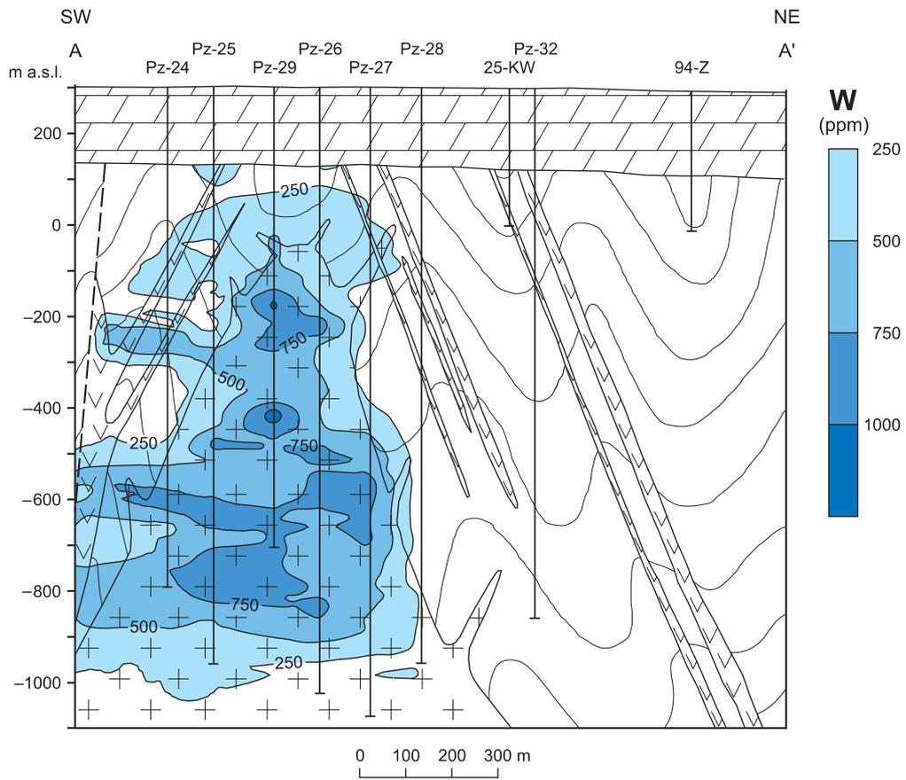
**Fig. 44. Tungsten content on the cross-section A-A'**
