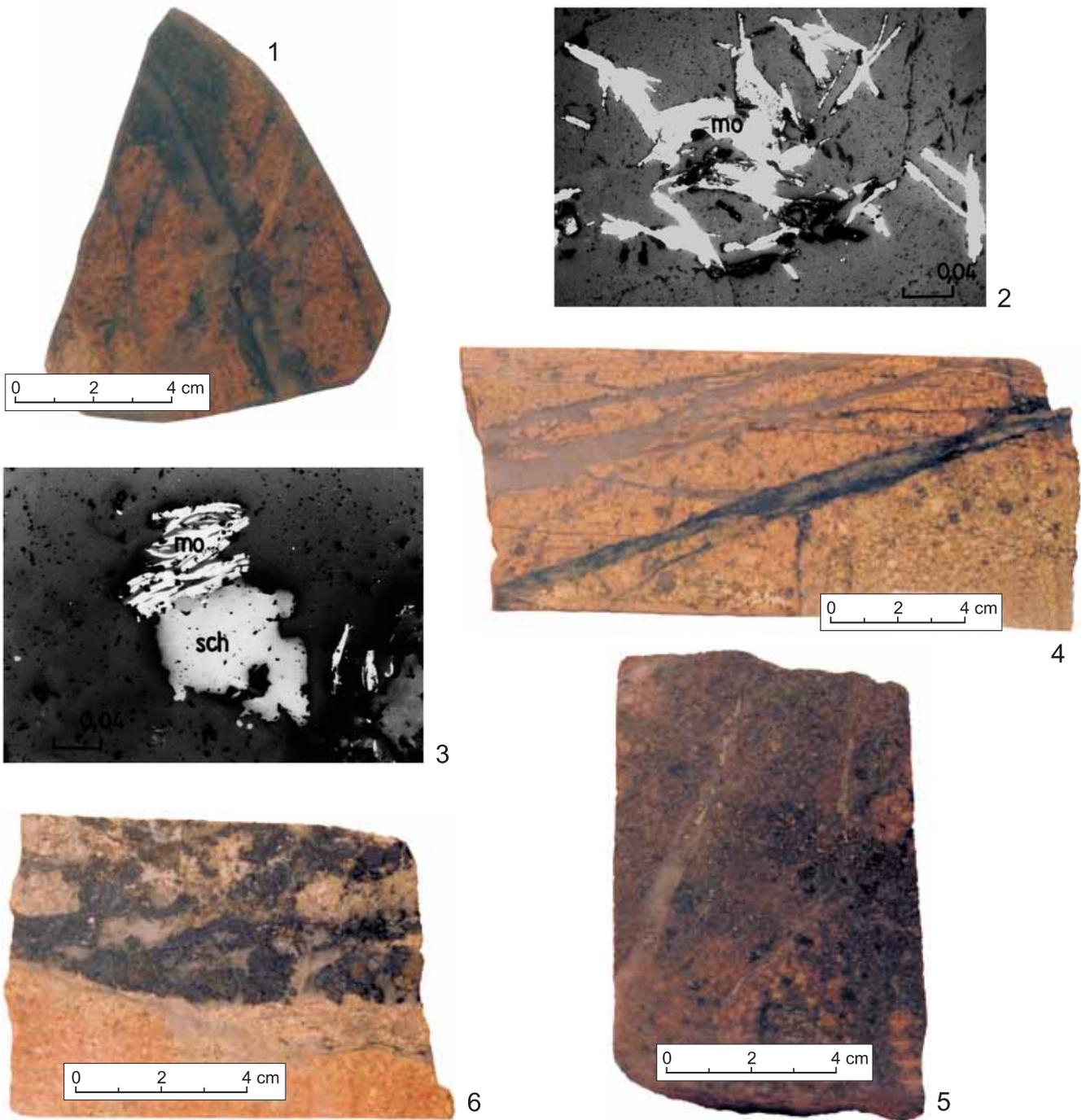
**Fig. 1.** Dark grey sericitised zone overlapping a deformed quartz vein. Pz-29/640.0 m.
