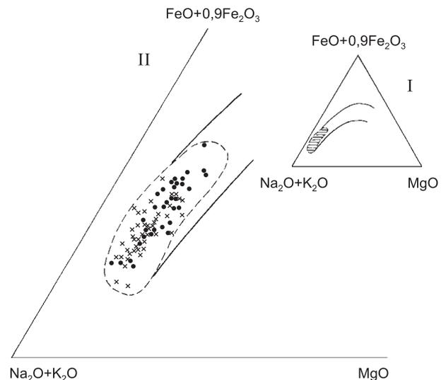
Fig. 27. Diagram (Na<sub>2</sub>O+K<sub>2</sub>O)–MgO–(FeO+0,9 Fe<sub>2</sub>O<sub>3</sub>) for magmatic rocks; after Masao *et al.*, 1965, supplemented by Markiewicz, 1998
