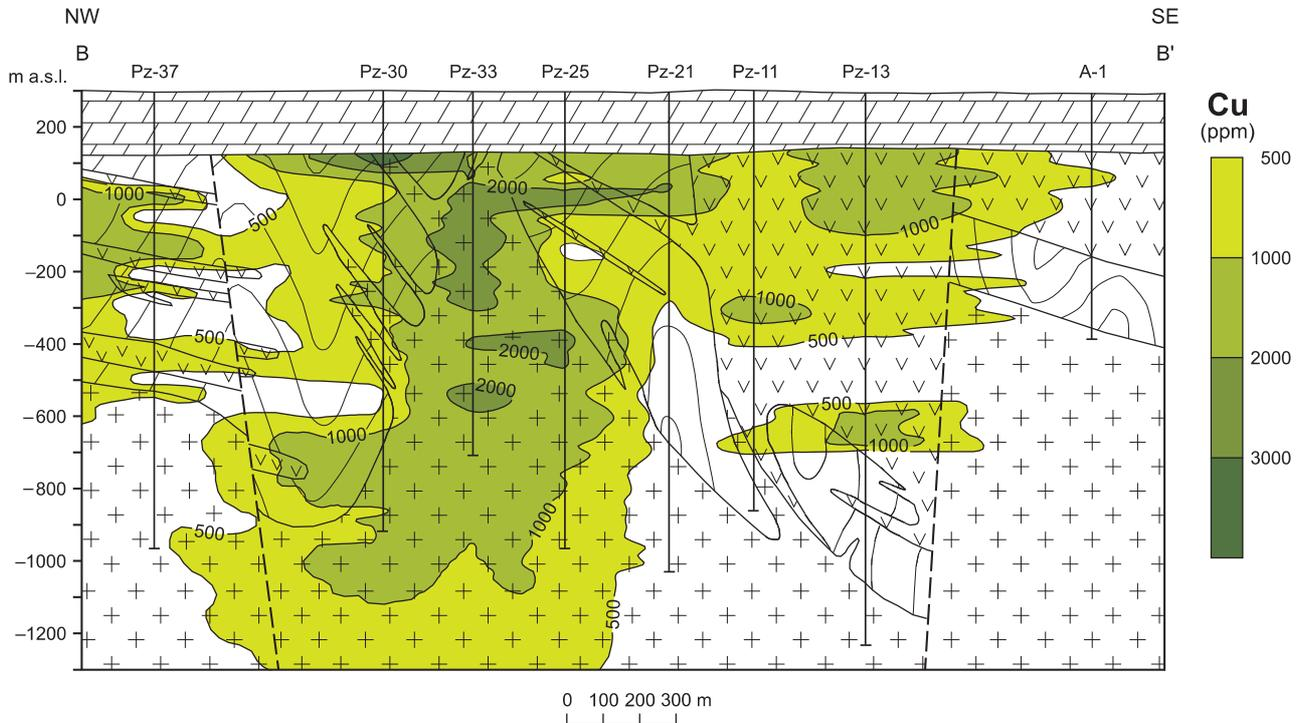
Fig. 47. Copper content on the cross-section B-B'
