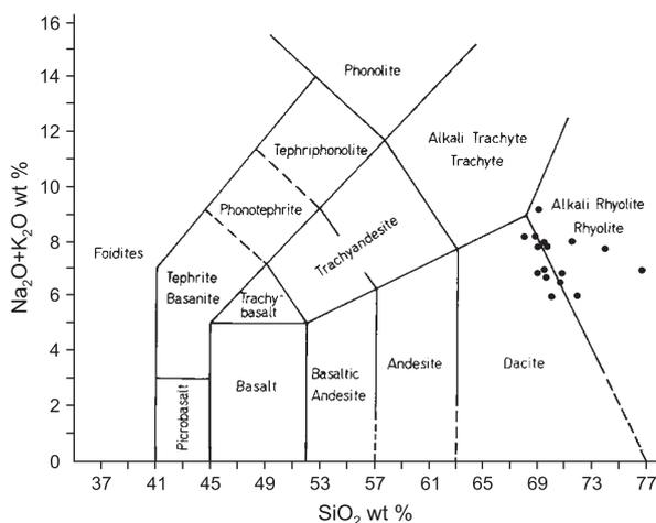
Fig. 26. TAS diagram (total alkali-silica) for dacitoids
