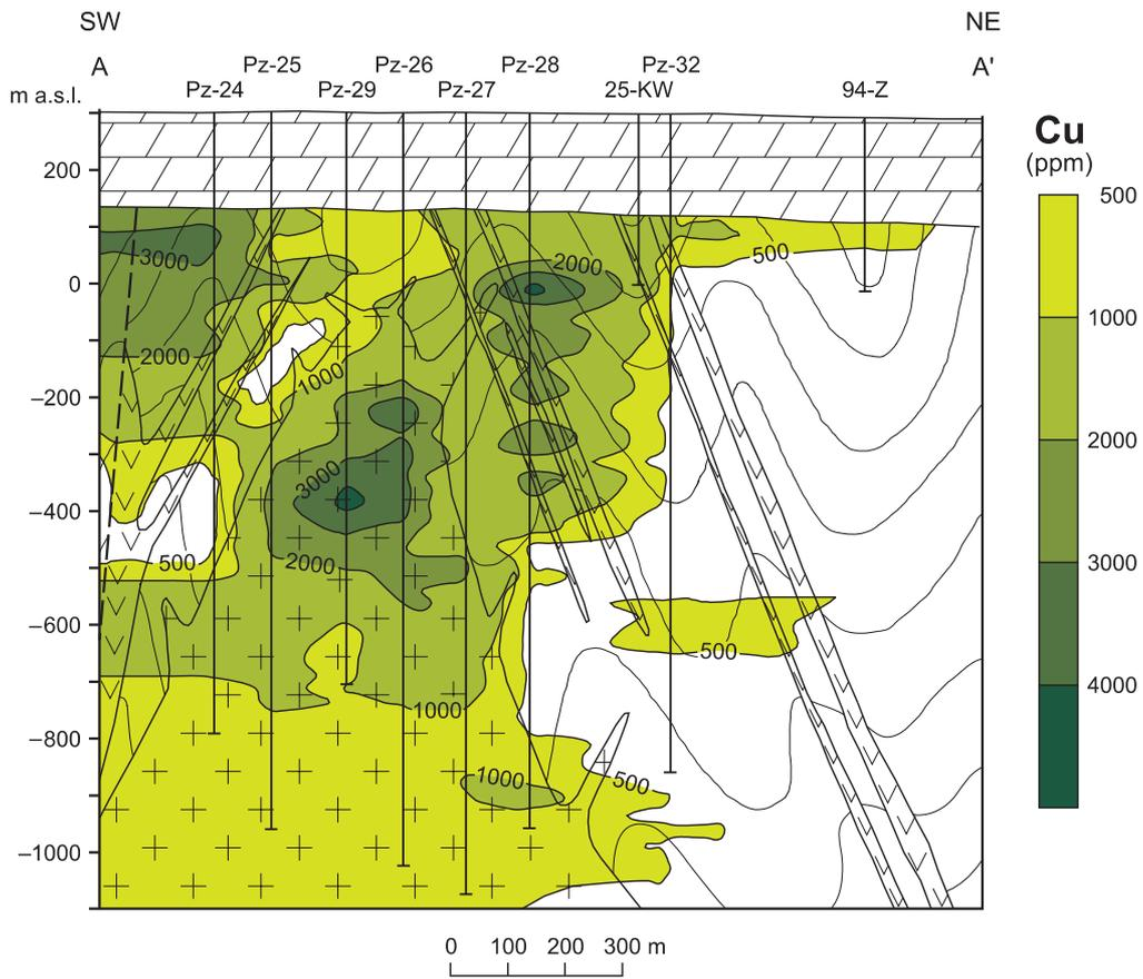
Fig. 46. Copper content on the cross-section A-A'
