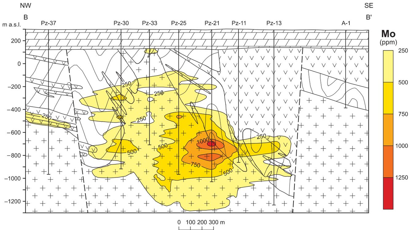
Fig. 43. Molybdenum content on the cross-section B–B’
