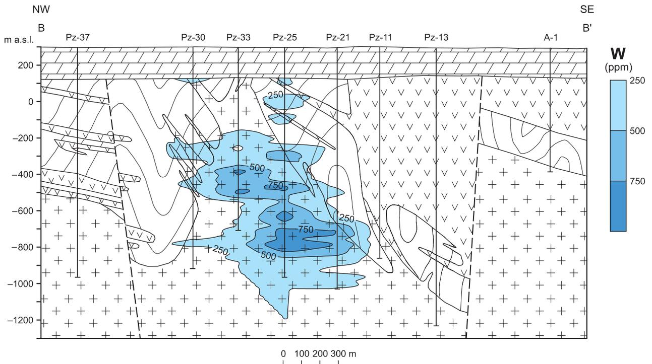
**Fig. 45. Tungsten content on the cross-section B-B'**
