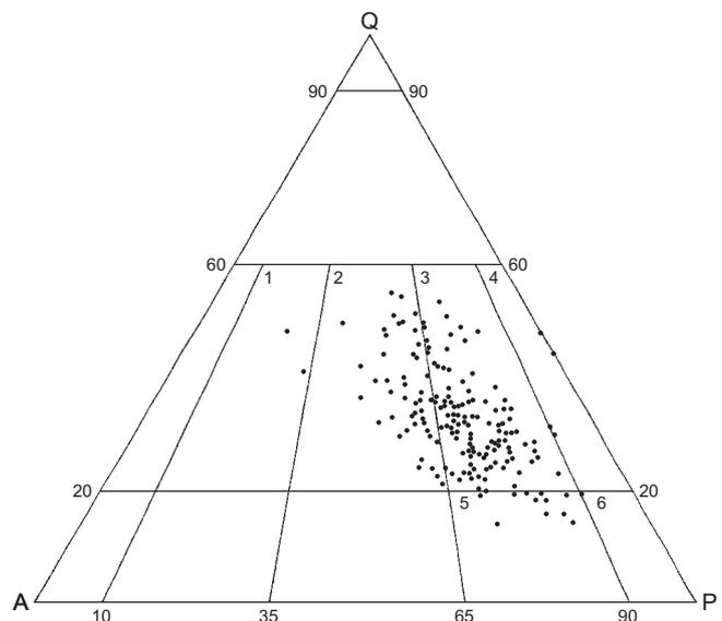
Fig. 20. QAP projection for granitoids, based on mineral content
