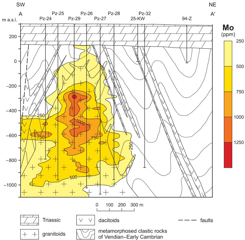
Fig. 42. Molybdenum content on the cross-section A–A’
