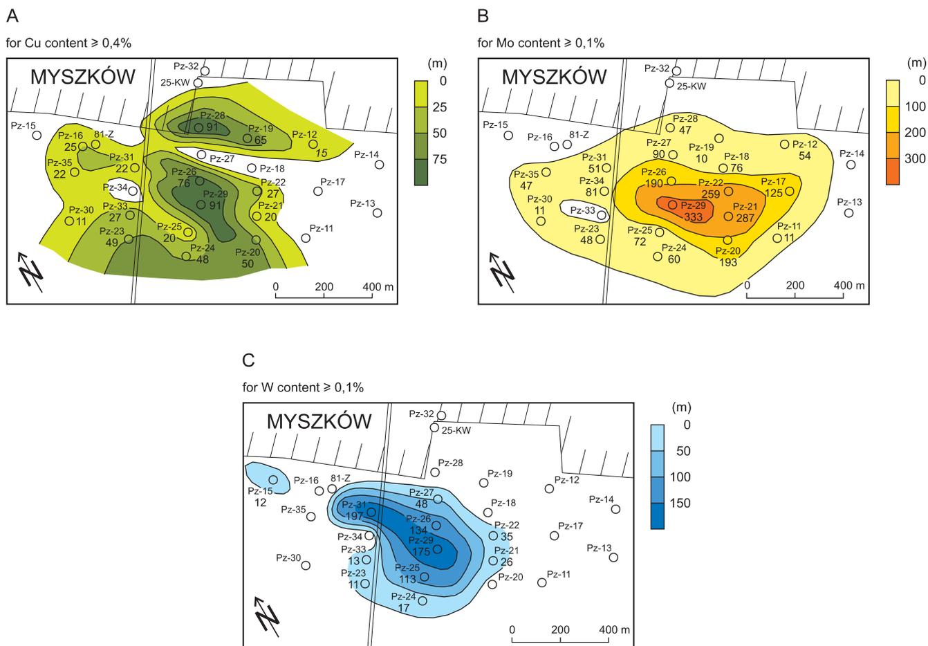
Fig. 48. Maps of the total mineralised intervals thickness of at least 10 m thick intervals
