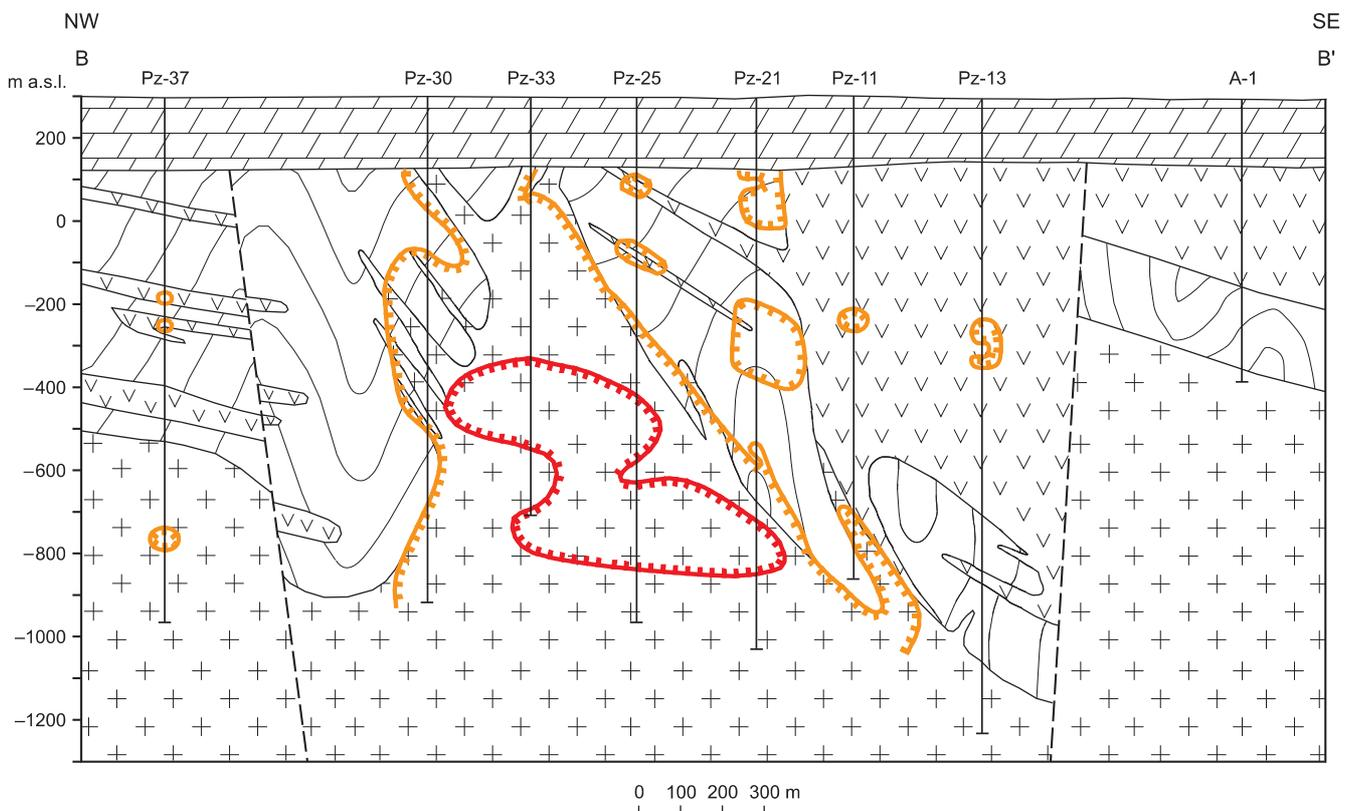
Fig. 40. Geochemical cross-section B-B': element related to felsic intrusive rock-associated mineralisation
