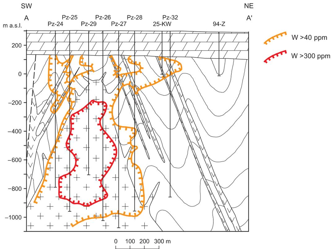
Fig. 39. Geochemical cross-section A-A': element related to felsic intrusive rock-associated mineralisation
