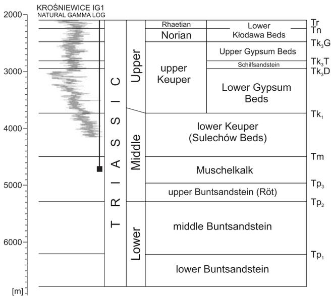
Fig. 3. Triassic lithostratigraphy (after Gajewska in: Marek and Pajchłowa, 1997, simplified) and the Triassic thickness distribution along and below the Krośniewice IG 1 borehole
