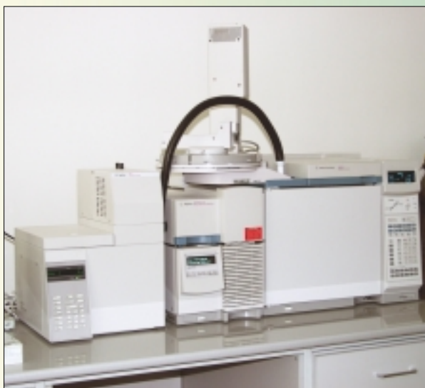
Chromatograf gazowy z detektorem masowym (GC-MSD) firmy Perlan Gas chromatograph with mass detector (GC-MSD) manufactured by Perlan
