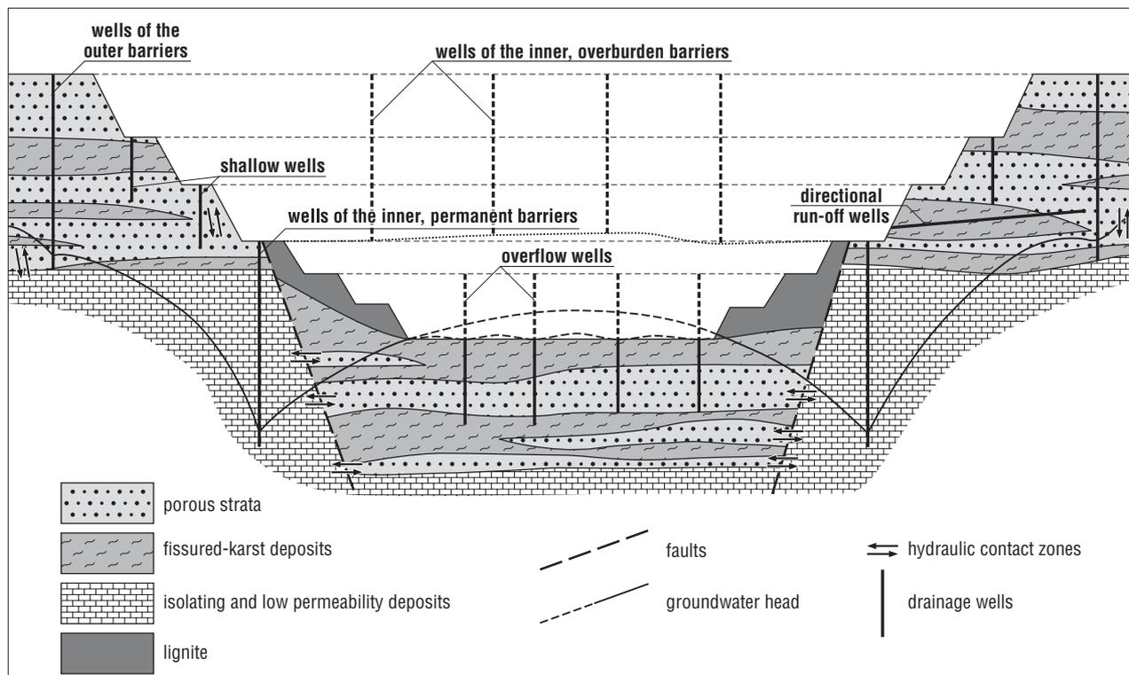
Fig. 5. Schematic diagram of the Bełchatów pit mine dewatering system (after Seweryn, 1984)
