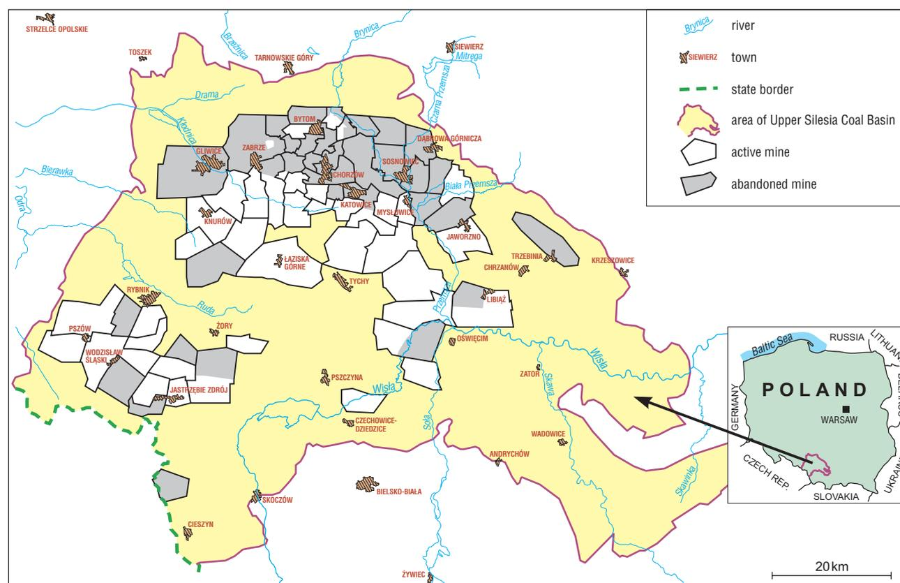
**Fig. 2. Locations of coal mining areas within the Upper Silesia Coal Basin (USCB), 2006**
