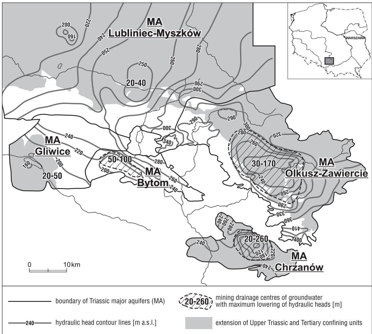
Fig. 6. Hydrogeological map of regional Triassic groundwater formation in the Zn-Pb mining area
