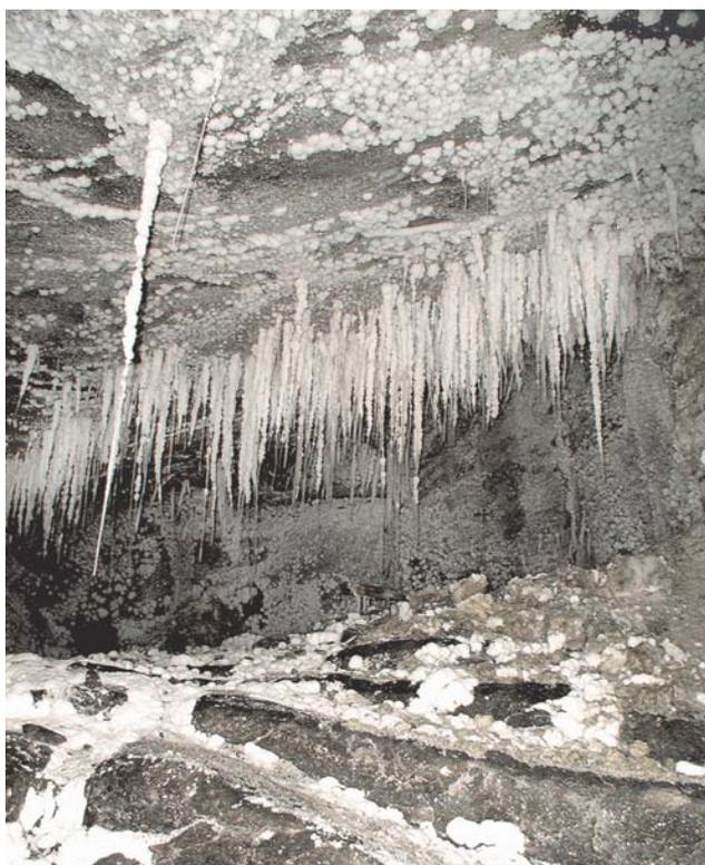
**Fig. 7.** Artificial dripstones in a Ferro chamber in the vicinity of the inflow WIIIn-19. Photo by J. Przybyło
