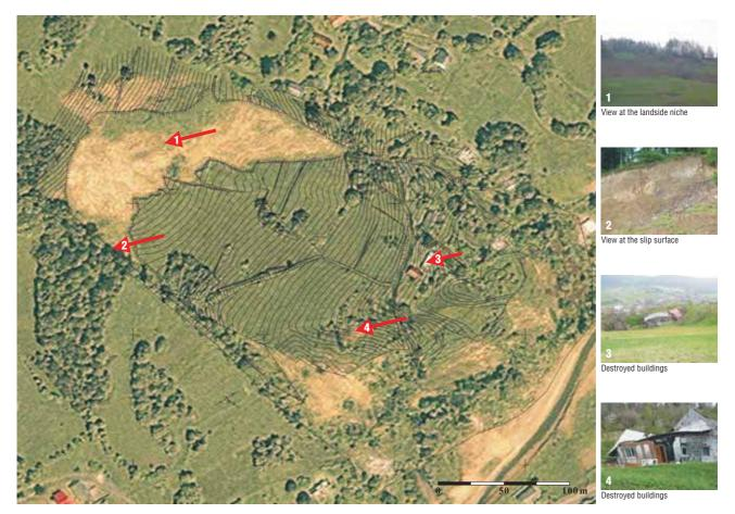
Fig. 3. The map showing the Lachowice landslide (compiled by Raczkowski in 1999) superimposed onto an IKONOS satellite image taken in 2002. The development of landslide activity and houses damages are clearly visible — indicated by arrows
