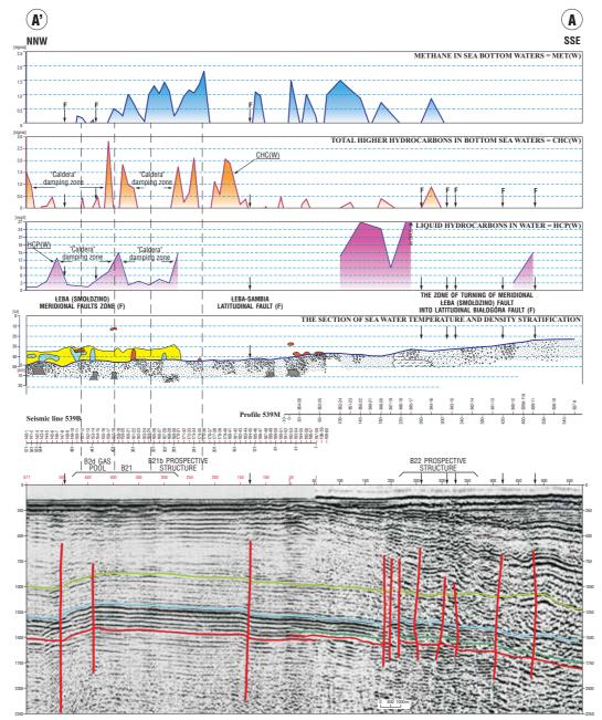
Fig. 2. Offshore geochemical-seismic profile A-A' (NNW–SSE) running from B21 gas-condensate deposit accumulated on hanging wall of the Smołdzino (Łeba) meridional fault to the tectonic crossing of the Smołdzino (Łeba) and the latitudinal Łeba–Sambia and Białogóra Fault
