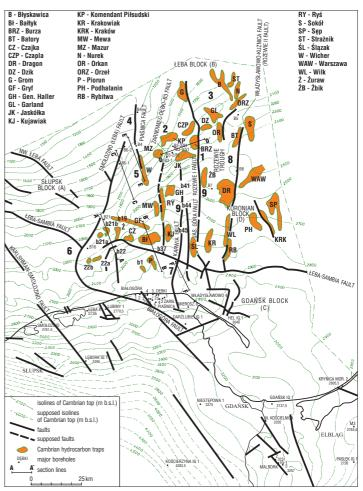
**Fig. 1.** Structure contour map of the Cambrian sediments and petroleum prospective zones as inferred from sea bottom geochemical studies correlated with subsurface geology from seismic profiles. Perspective zones were given the names of former warships of the Polish Navy
