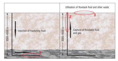
Fig. 6. A scheme of theoretical routes of pollutants migration (1 - from the horizontal section of well, 2 - from the near-well zone of its vertical section, 3 - from the surface)
