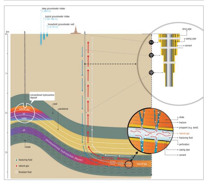
Fig. 3. A scheme of hydrauling fracturing process
