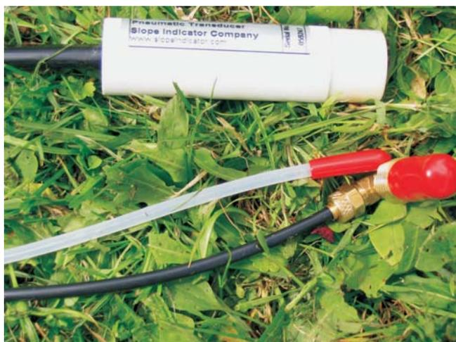
Fig. 19. Pneumatic piezometer transducer
