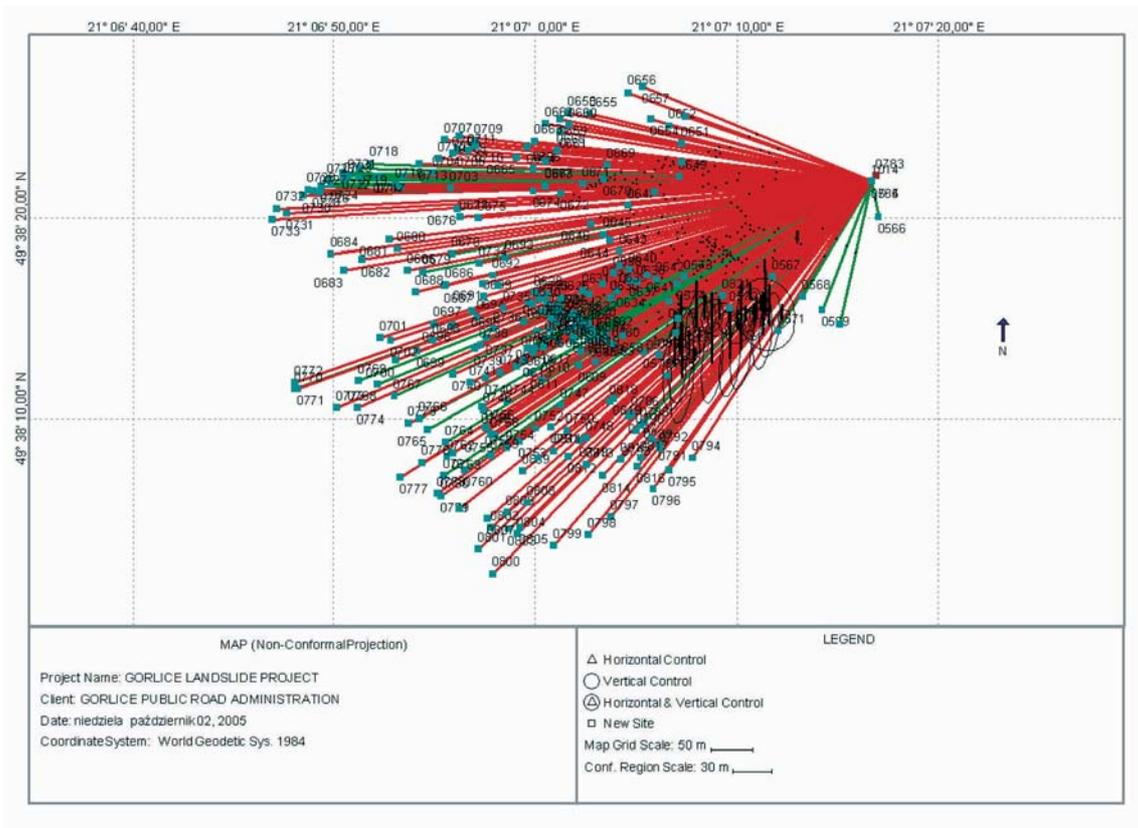
Fig. 6. Bystrzyca landslide morphology modelling using GPS measurements
