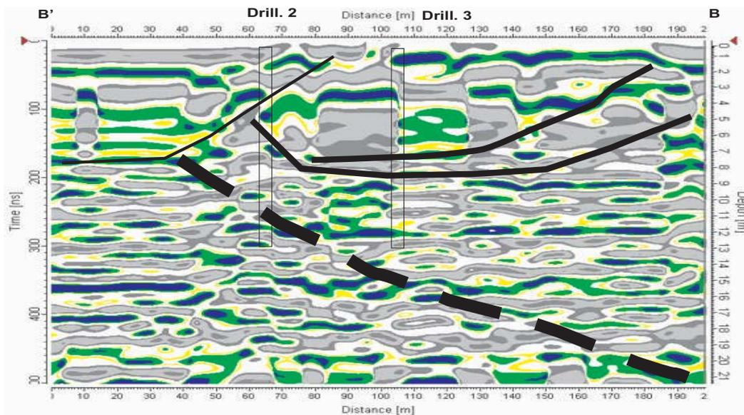
Fig. 11. GPR B'-B longitudinal scanning profile, Sękowa landslide
