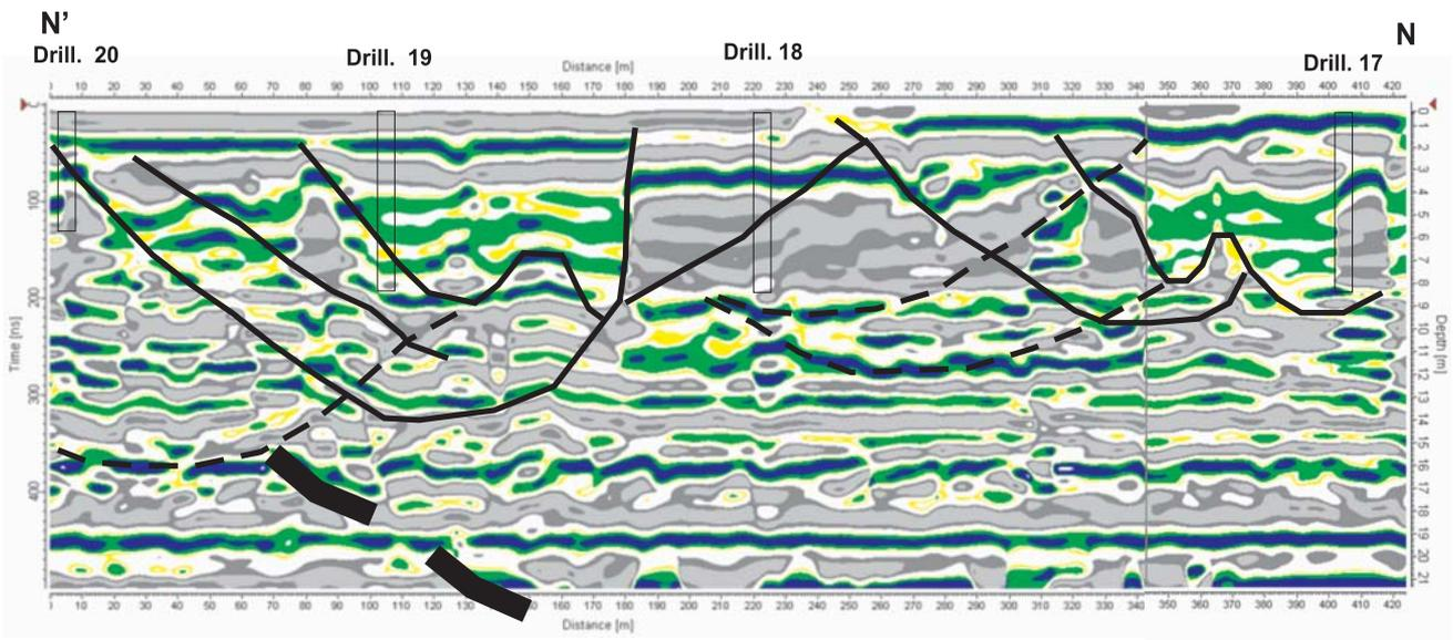
Fig. 10. GPR N-N' transverse scanning profile, Wapienne landslide
