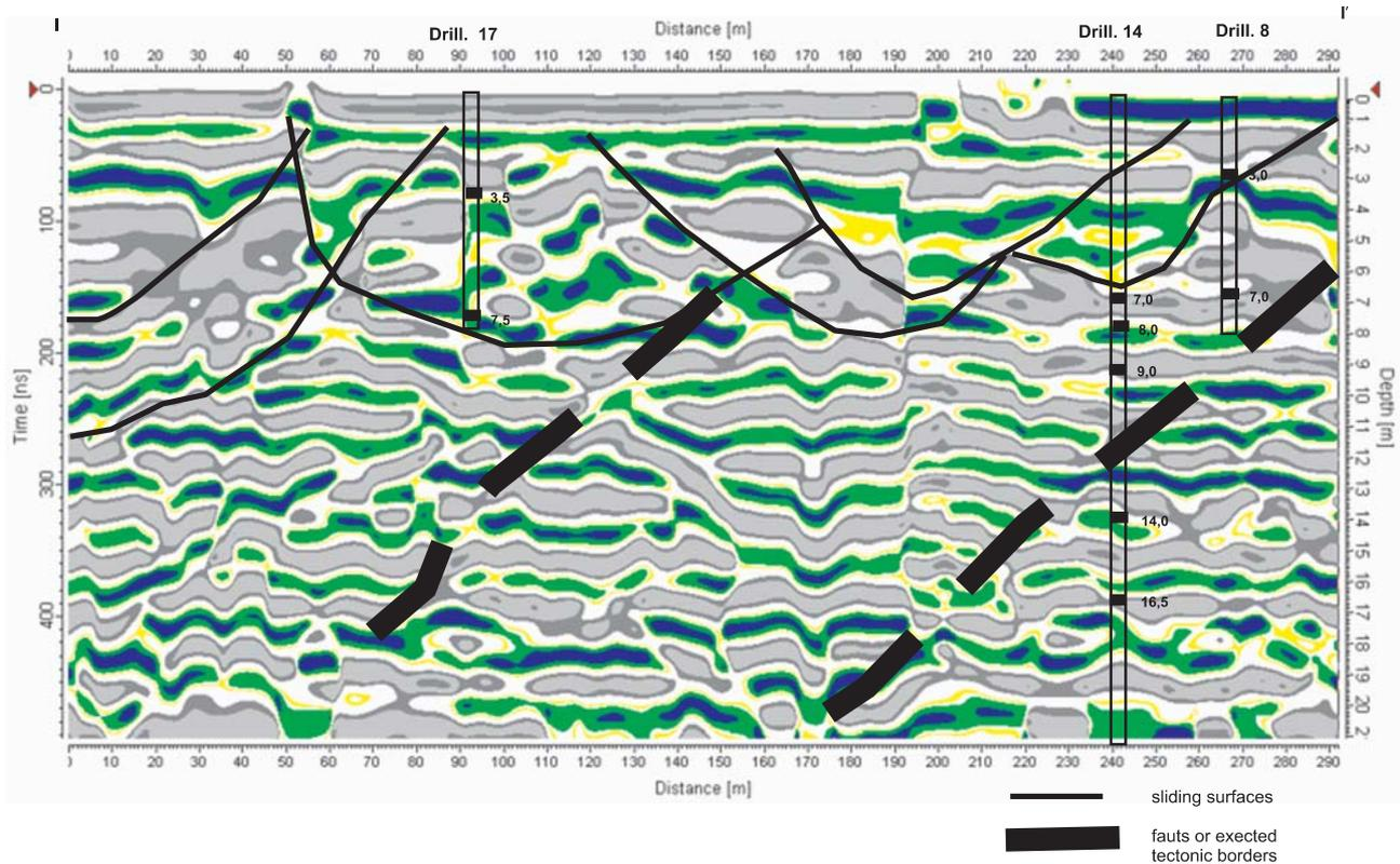
Fig. 9. GPR I-I' longitudinal scanning profile, Wapienne landslide
