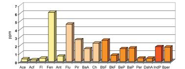
Fig. 4. Polycyclic aromatic hydrocarbons in soil from "Przyjaźń" coking plant area
