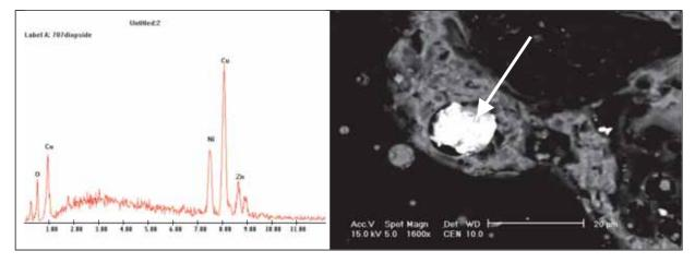
b) SEM image with EDS spectrum of aluminosilicate particles containing copper
