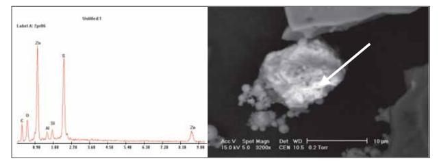
Fig. 1. Examples of the fly ash particles containing heavy metals
