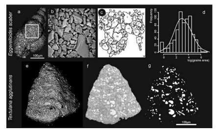
Grain shape characterization. Global **SEM** backscattered electrons (BSE) image of a specimen of Eggerelloides scaber; SEM BSE image of the selected surface for grain analysis, c) Separation of grains that are entirely observed within the selected area and calculation of the parameters; shape Distribution of surface of grains (log). Log-normal curve is superimposed. e) Example of quartz analysis
