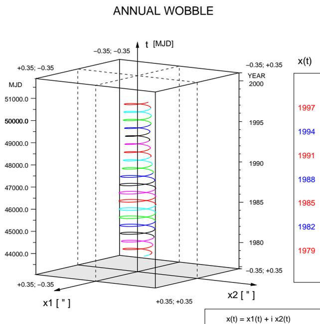
**Figure 3.** Annual wobble filtered out from the series EOP (JPL) SPACE99 using the mathematical perspective in space-time view of Höpfner (1994a). The  $x_1$ -axis points towards the Greenwich meridian and the  $x_2$ -axis towards  $90^0$  E longitude.
