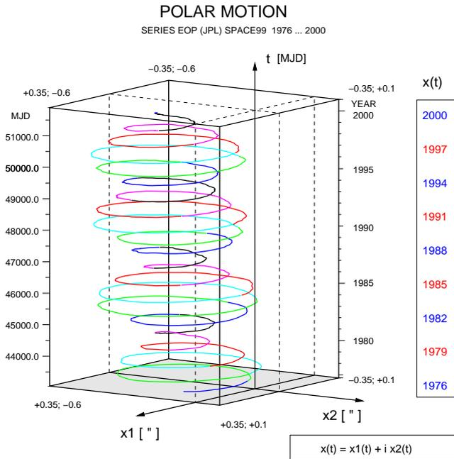
**Figure 1.** Polar motion as computed by JPL (Gross, 2000) using the mathematical perspective in space-time view of Höpfner (1994a). The  $x_1$ -axis points towards the Greenwich meridian and the  $x_2$ -axis towards  $90^\circ$  E longitude.
