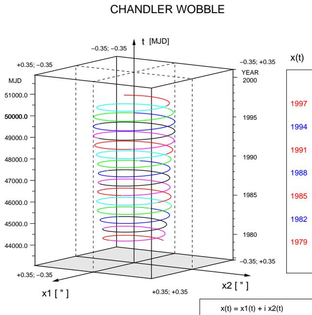
**Figure 2.** Chandler wobble filtered out from the series EOP (JPL) SPACE99 using the mathematical perspective in space-time view of Höpfner (1994a). The  $x_1$ -axis points towards the Greenwich meridian and the  $x_2$ -axis towards  $90^0$  E longitude.
