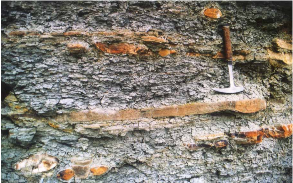
Figure 3-20: Glauconitic shale (shale lithofacies) with lenticular sandy storm beds and oval mudstone cobbles in the Redwater Shale Member at section Flaming Gorge (FG). Hammer is 32 cm long.
