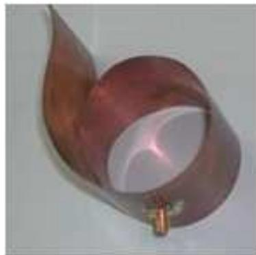
Figure 2.4: Fabricated prototype of the proposed antenna with SMA feed..
