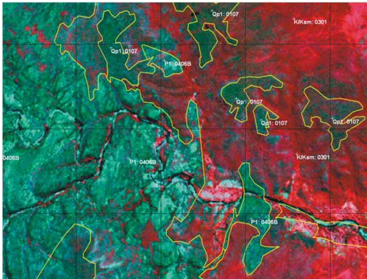
Fig. 3. Image interpretation of an ASTER VNIR scene at ca. 23°25' S and 31°50' E. The interpretation shows isolated outcrops of Umbelúzi rhyolite (Karoo Supergroup) east of its main boundary with the Cretaceous Grudja Formation. Note the isolated pockets of Quaternary cover (Qp1) covering the Grudja Formation (K/Ksm). Grid lines are north-oriented and spaced 2 km apart.
