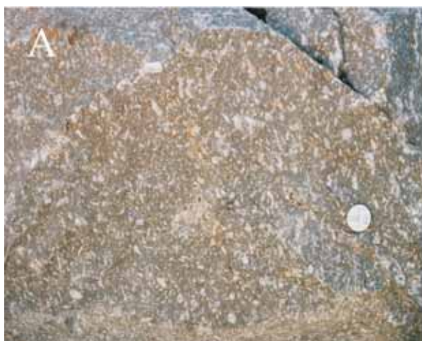
Fig. 13. a) Porphyritic texture of the Pessene nepheline syenite. b) Photomicrograph of nepheline syenite, with euhedral phenocrysts in a microcrystalline ground mass. X-nicols. The Pessene quarry (0431268/7150433). Coin diameter 2.5 cm, photo width 3.5 cm.
