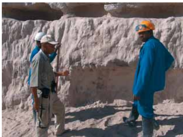
Fig. 5. Diane quarry, exploiting a one-metre-thick diatomite layer (in the middle of the picture), Manhiça (SDS 2532, 463968/ 7193482).
