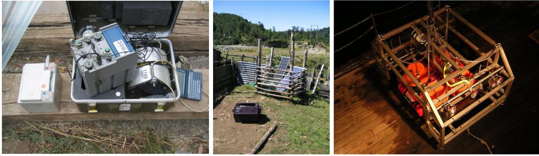
Figure 3.3: Left: EDL station with battery, datalogger and Mark L4-3D seismometer and external service unit. Middle: EDL station deployment with solar panels and additional fence against animals. Right: OBS station.
