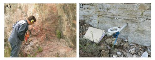
**Fig. 2.** (A) Sampling at Rajamäki with the gasoline drill. (B) Core orienting with sun and magnetic compass at Kallasto.
