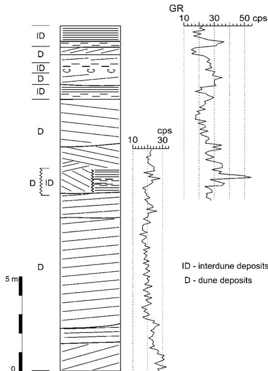
Fig. IV.2.2. Interbedding of dune and interdune deposits in the Tumlin-Gród quarry and its  $\gamma$ -ray pattern.
