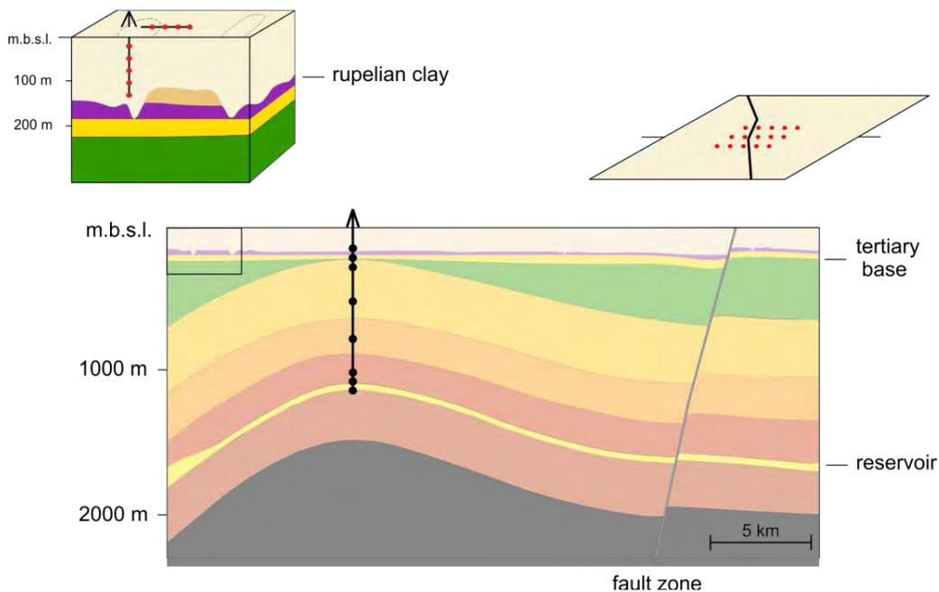
**Fig. 1:** Concept of a monitoring system including combined surface-downhole measurements near the formation defects, an adapted electrode array in the wellbore and parallel profiles along the fault zone (f.l.t.r.).
