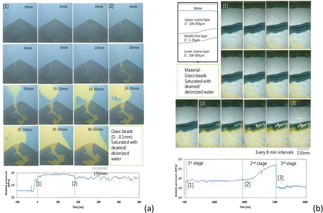
**Fig. 2:** The results of CO<sub>2</sub> gas injection test (time-lapse digital images and time history of gas bubble pressure): (a) a sea bottom mountain model, (b) a layered glassbead-water mixture system having a fine middle layer.
