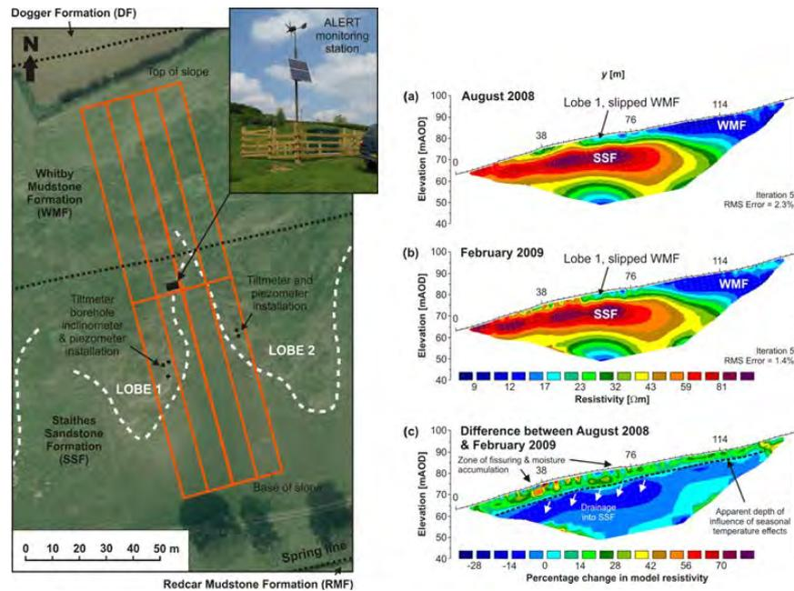
**Fig. 4:** Left: location of the ALERT station and ERT monitoring arrays (red lines); right: (a) August 2008 and (b) February 2009 ERT models, and (c) resulting differential resistivity image (modified from CHAMBERS et al., 2009).
