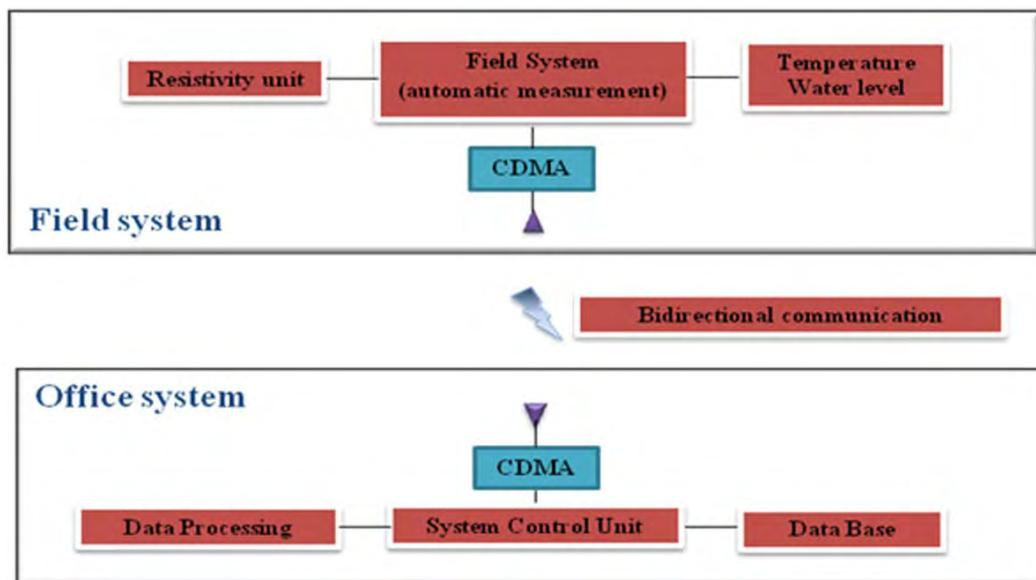
Fig. 4: Resistivity monitoring system devised for the leakage detection in embankment dams.
