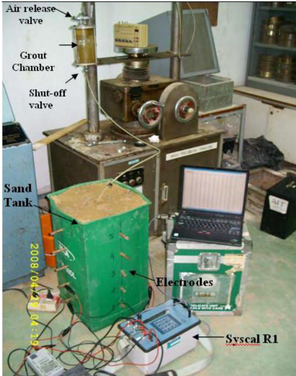
**Fig. 12:** View of the grouting and ERT setup.
