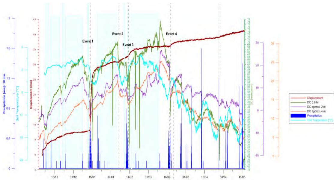
**Fig. 7:** Display of displacement (red), precipitation (blue; courtesy of the Central Institute for Meteorology and Geodynamics (ZAMG)) and apparent resistivity at different relative apparent depths (green: 1 m; purple: 2 m; orange: 4 m) in the winter/spring period.
