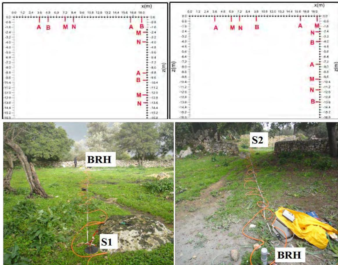
**Fig. 3:** (up) Dipole-Dipole (left) and gradient (right) electrode configurations for the surface, borehole and surface-to borehole measurements. (down) Arrangement of the surface electrodes along the lines S1 - BRH and S2 - BRH, where BRH shows the location of the borehole.
