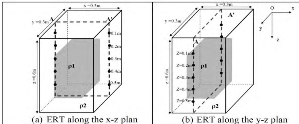
Fig. 7: Simulation of ERT monitoring on the synthetic grouting model.
