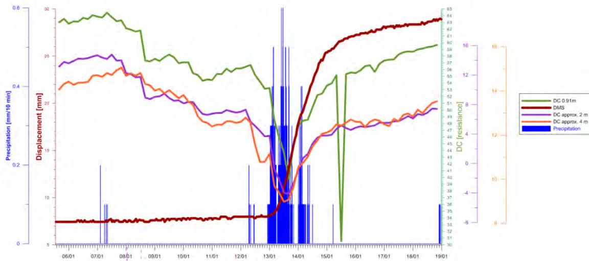
**Fig. 8:** Display of displacement (red), precipitation (blue; from the station Wolfsegg, courtesy of the Central Institute for Meteorology and Geodynamics (ZAMG)) and apparent resistivity at different relative apparent depths (green: 1 m; purple: 2 m; orange: 4 m) for the time around the major displacement event (“event1”) in January 2011.
