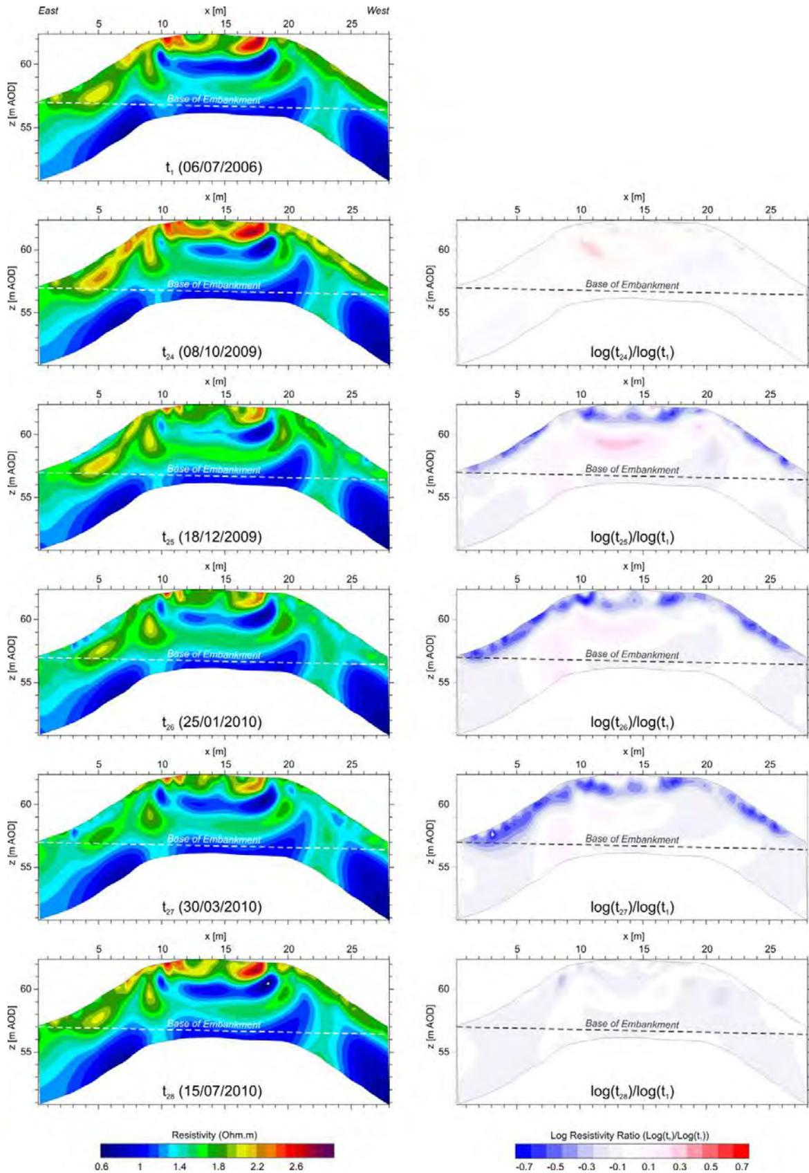
**Fig. 6:** Temperature corrected 2D ERT model sections (left) and log resistivity ratio plots (right) showing changes in resistivity relative to the July 2006 baseline (top left).
