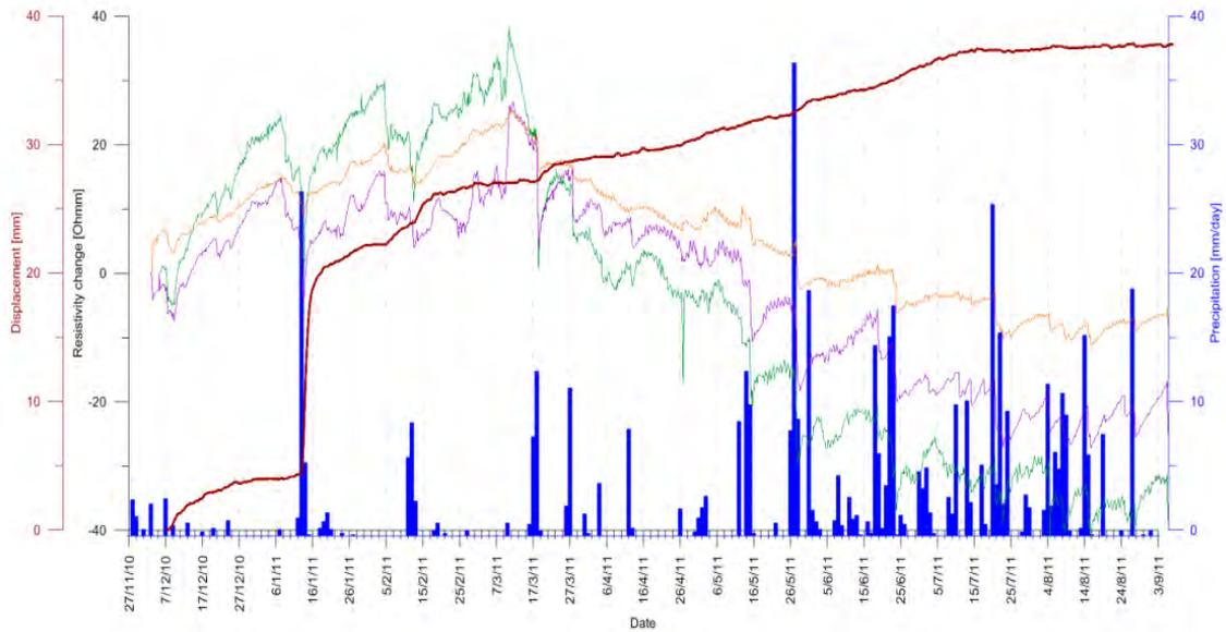
**Fig. 6:** Display of displacement (red), precipitation (blue; courtesy of the Central Institute for Meteorology and Geodynamics (ZAMG)) and apparent resistivity at different relative apparent depths (green: 1 m; purple: 2 m; orange: 4 m) for the whole survey period.
