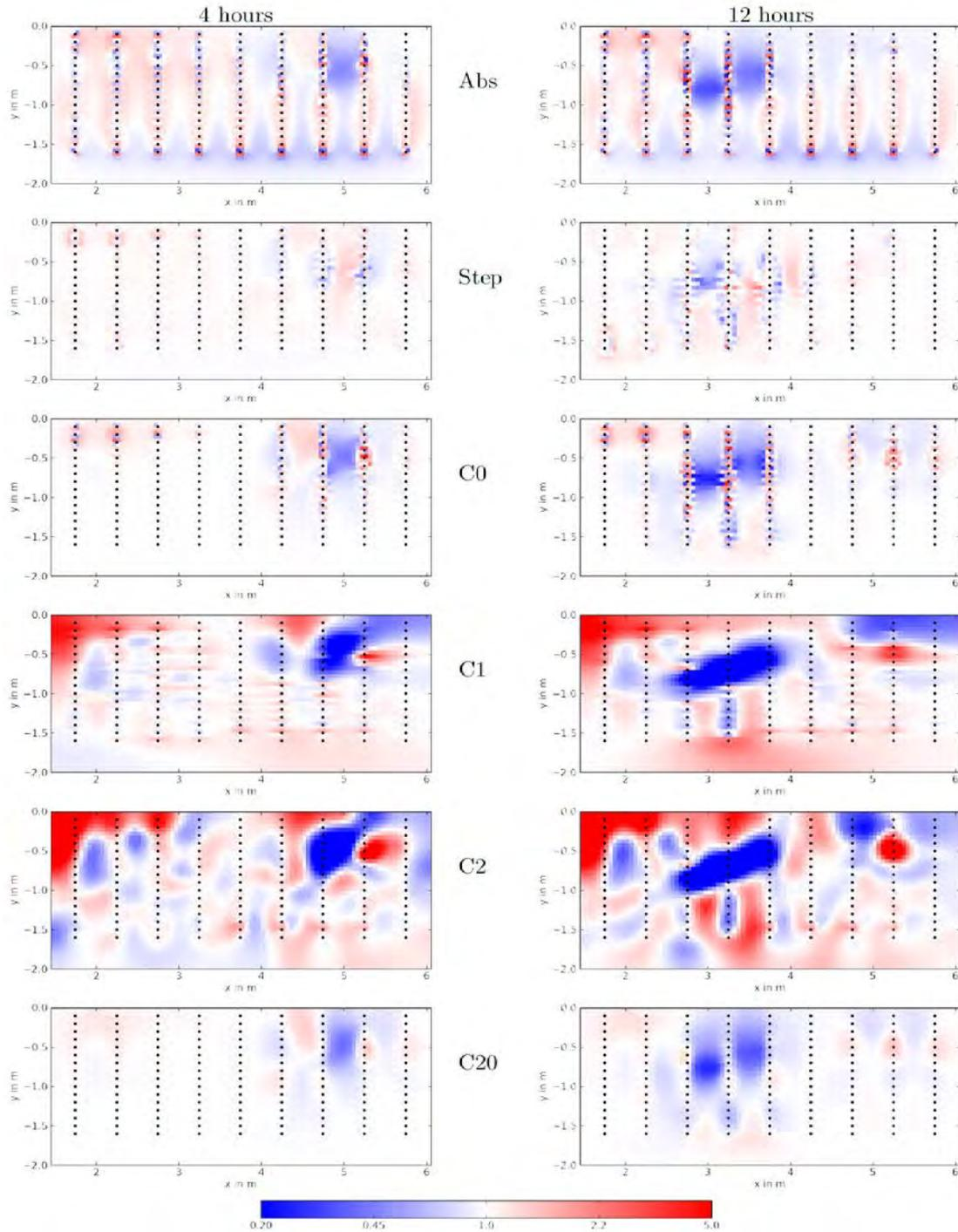
**Fig. 6:** Resistivity ratio for timesteps 4 hours (left) and 12 hours (right) and inversion schemes: individual inversion, step-wise constrained and difference inversion using constraint orders 0, 1, 2 and 0+2.
