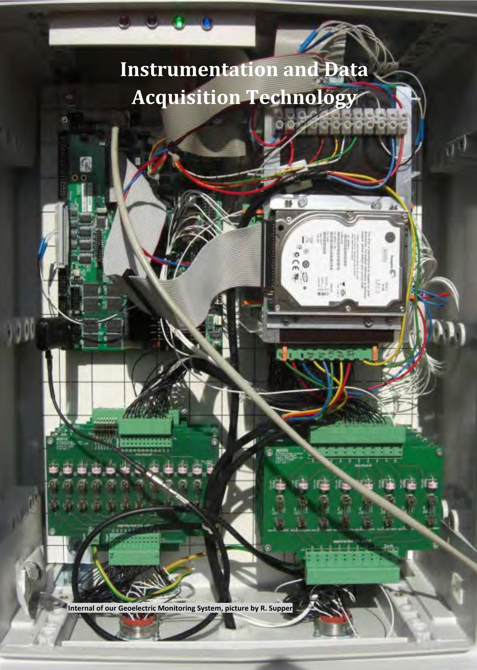
Internal of our Goelectric Monitoring System, picture by R. Supper
