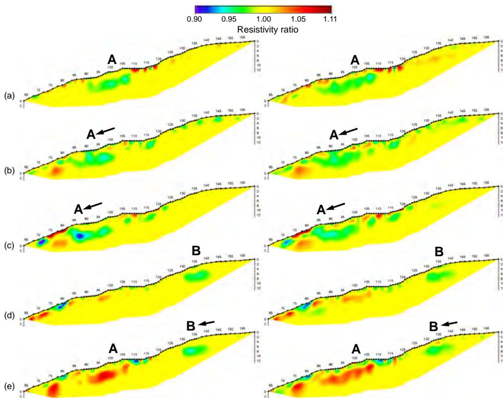
**Fig. 4:** Reconstructed difference images between two sequential time steps. The left column is the results by the L2D\_L2S\_L1T approach while the right is L2D\_L2S\_L2T. (a) T3/T2. (b) T4/T3. (c) T5/T4. (d) T6/T5. (e) T7/T6.
