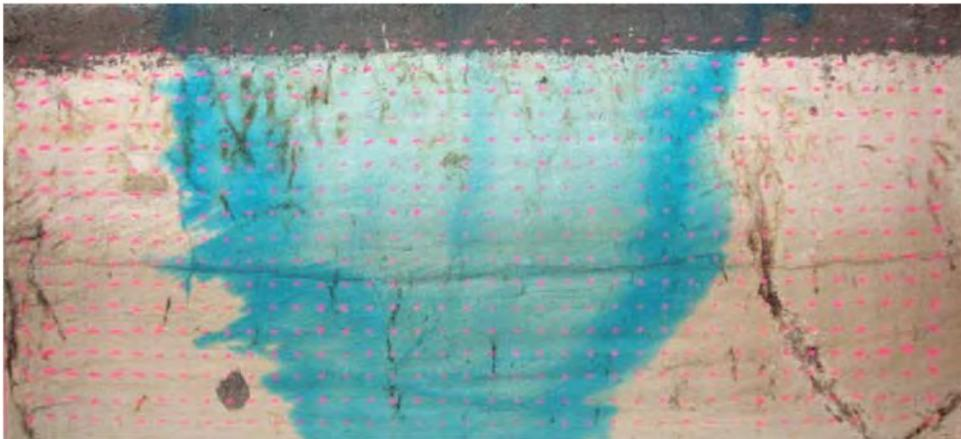
Fig. 4: Picture of the central section with blue infiltration plume
