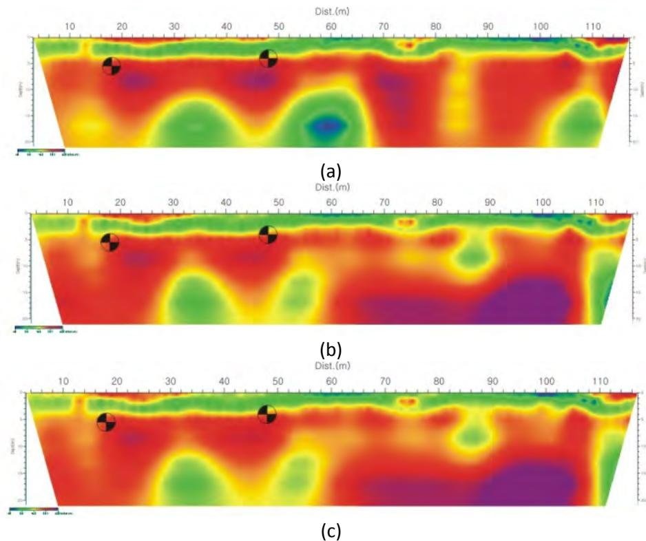
**Fig. 2:** Time-lapse images of electrical resistivity survey of Phase 0 in the crest (a), and the measurement of Phase 2 (b), and when Phase 9 measurement was completed (c).
