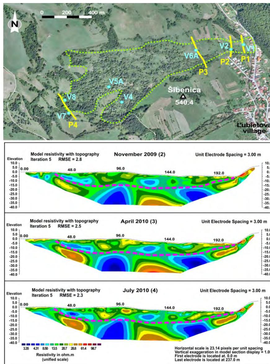
Fig.1: ERT monitoring on the Ľubietová active landslide.
