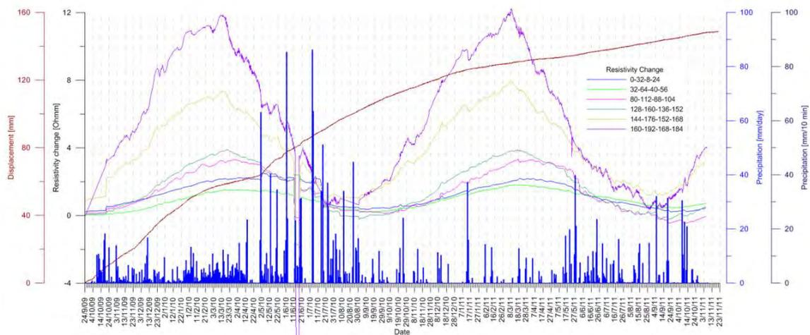
**Fig. 3:** Correlation of selected apparent resistivity data with displacement and precipitation for the entire survey period.
