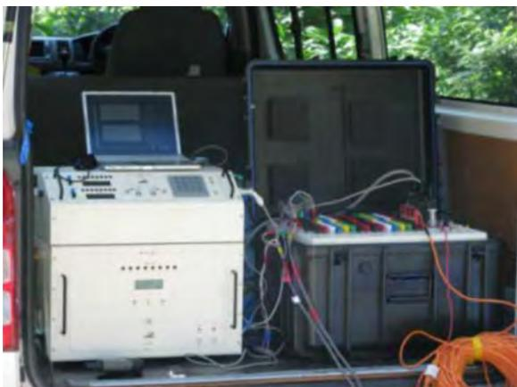
Fig. 5: A photo of multi-transmission resistivity meter.
