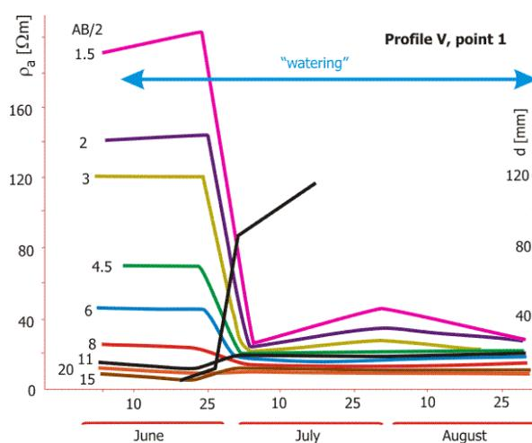
Fig. 7 Changes in apparent resistivity with moistening
