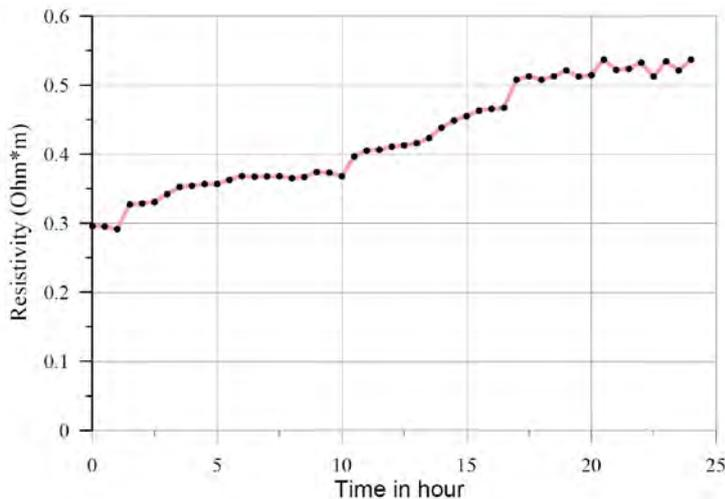
**Fig. 4:** Resistivity of grouting material vs. time.
