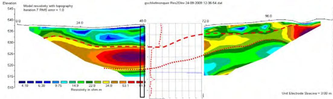
**Fig. 2:** Correlation of resistivity layers with sliding surfaces determined by a permanent inclinometer (red curve) in the area of Gschlietgraben.
