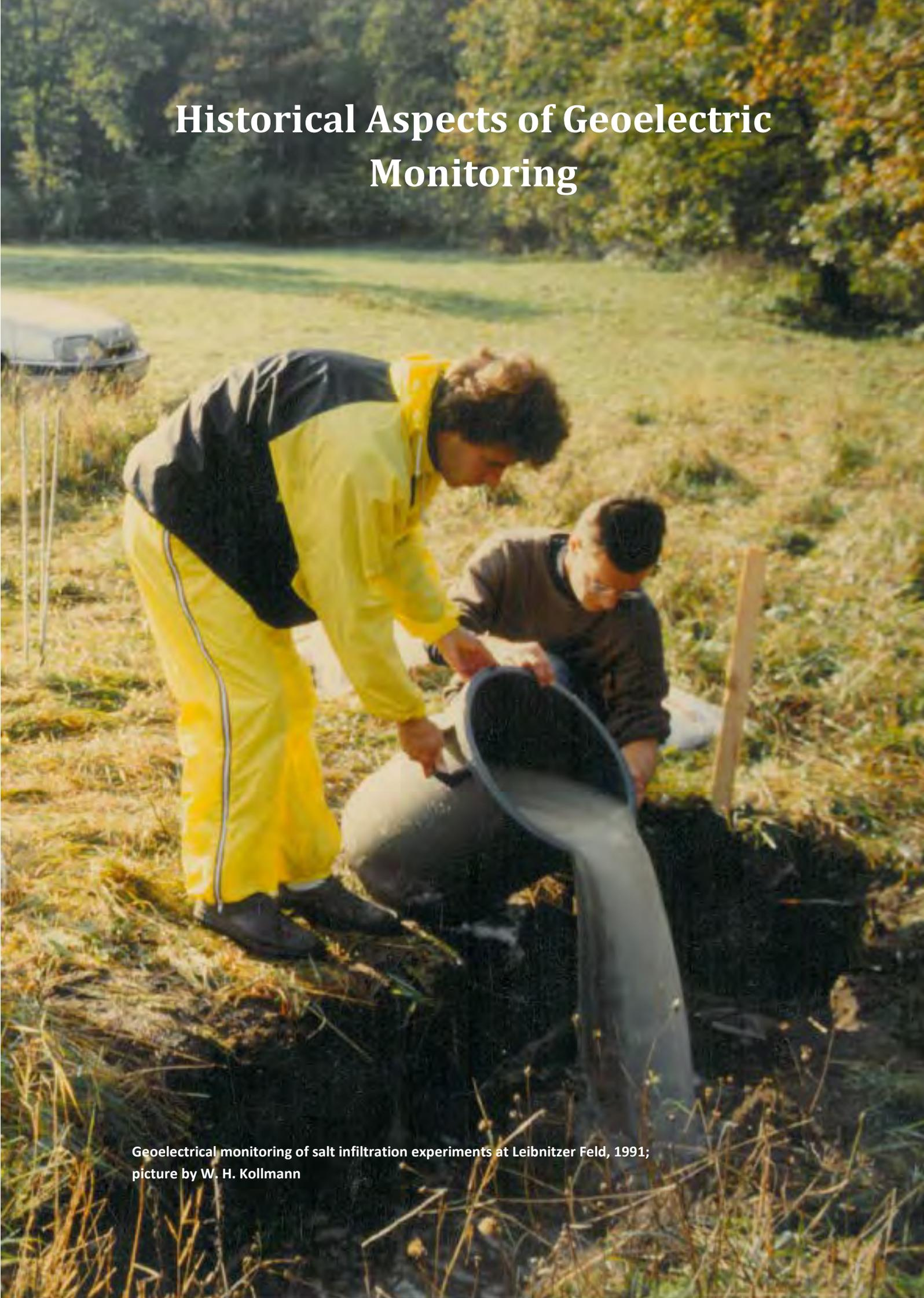
Geoelectrical monitoring of salt infiltration experiments at Leibnitzer Feld, 1991;
