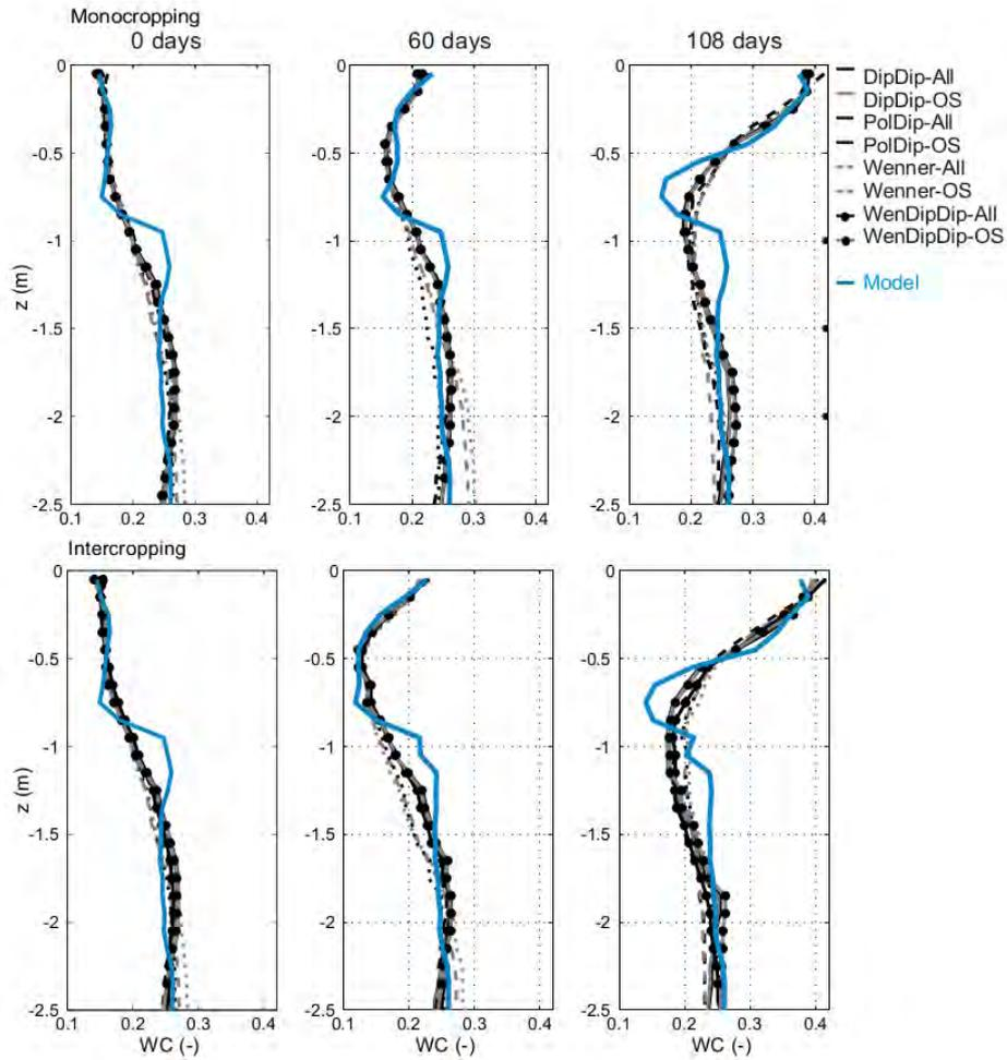
**Fig. 2:** 1-D water content profiles for the mono- and intercropping case at  $t = 0, 60$  and  $108$  days for a profile of  $2\text{m}$  width and  $3\text{m}$  depth in the middle of the simulated domain. The simulated values are represented by the thick, blue line. DipDip = dipole-dipole, PolDip = pole-dipole, WenDipDip = combination of Wenner & Dipole-dipole. Electrode arrays using only surface electrodes are marked by OS.
