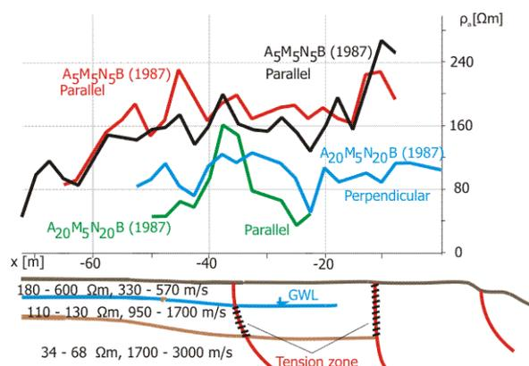
Fig. 5 Resistivity profiling on the landslide Trinec
