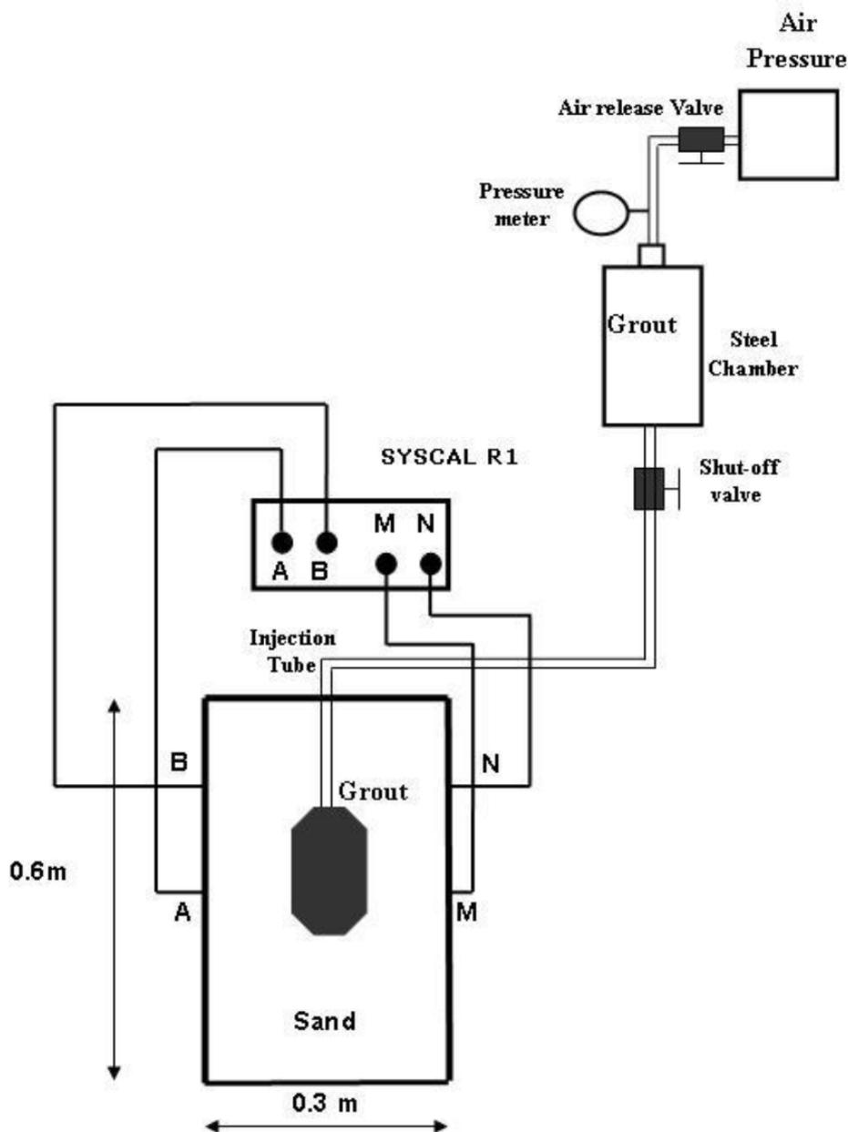
Fig. 11: Setup of grouting and ERT test.
