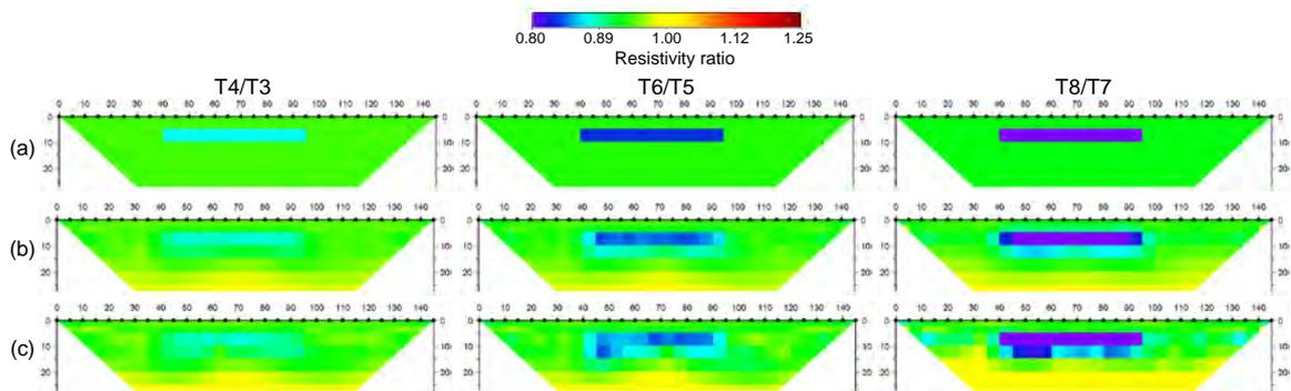
**Fig. 3:** Inversion experiments based on the test model of Figure 2. (a) The true model changes between sequential time steps. (b) L2D\_L2S\_L1T. (c) L2D\_L2S\_L1T. Regularization parameters were automatically determined.
