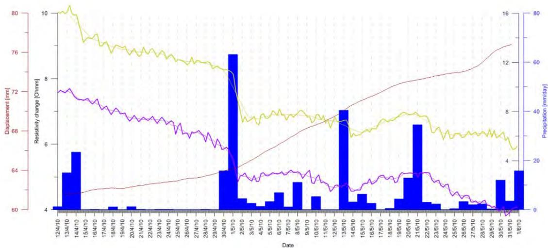
**Fig. 4:** Correlation of selected apparent resistivity data (yellow, purple) with displacement and precipitation for the event on March 1<sup>st</sup>, 2010.
