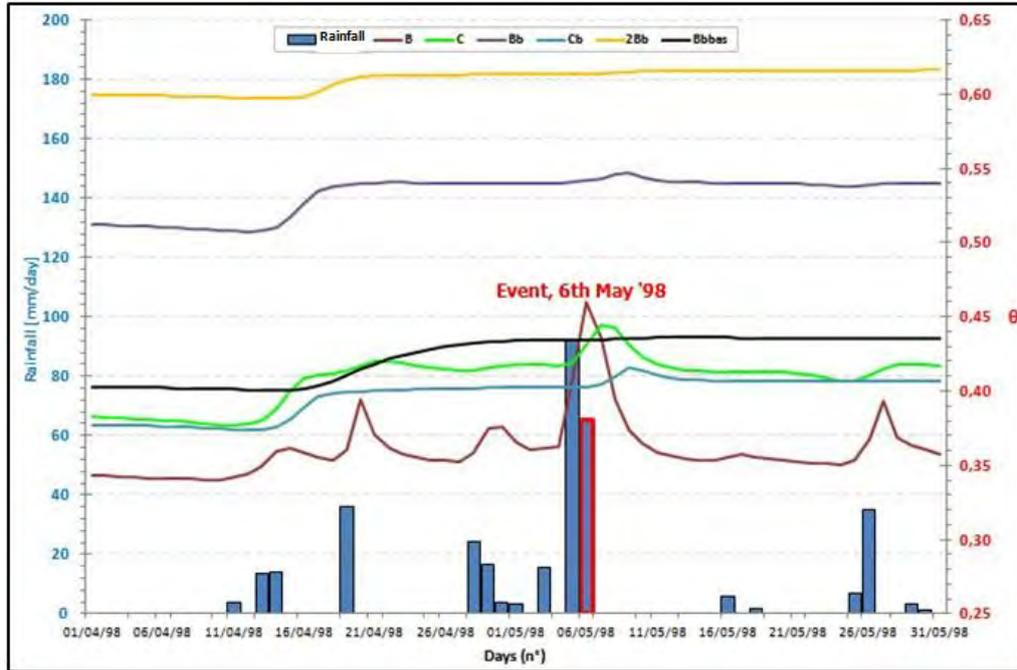
**Fig. 4:** Water content ( $\theta$ ) vs. time for each layer of the pyroclastic cover. The curves are correlated with the daily rainfall histograms (blue rectangles). The rectangle marked with the red edge indicates the rainfall occurred on May 6<sup>th</sup>, 1998.
