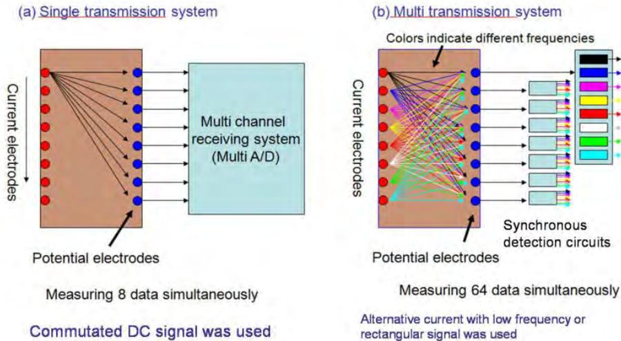
Fig. 1: Comparison of conceptual diagrams of the systems.
