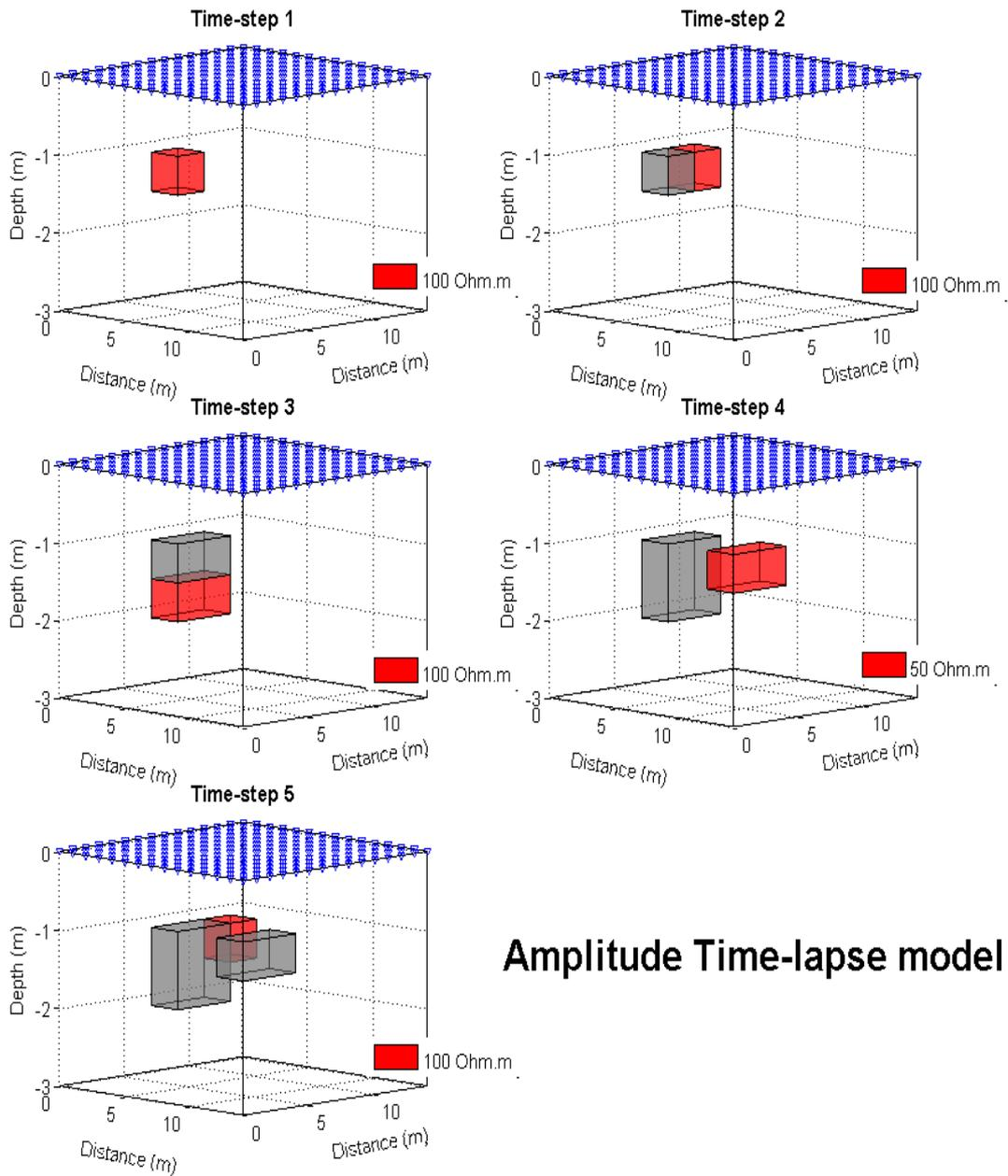
**Fig. 1:** The 4D resistivity model used in this work showing the changes in amplitude through time (five time-steps). The grey cubes denote the synthetic model used in the previous time-step. The red cubes show the change in that time-step with respect to the previous time-steps. The background model has a constant resistivity amplitude of 10  $\Omega$ m.
