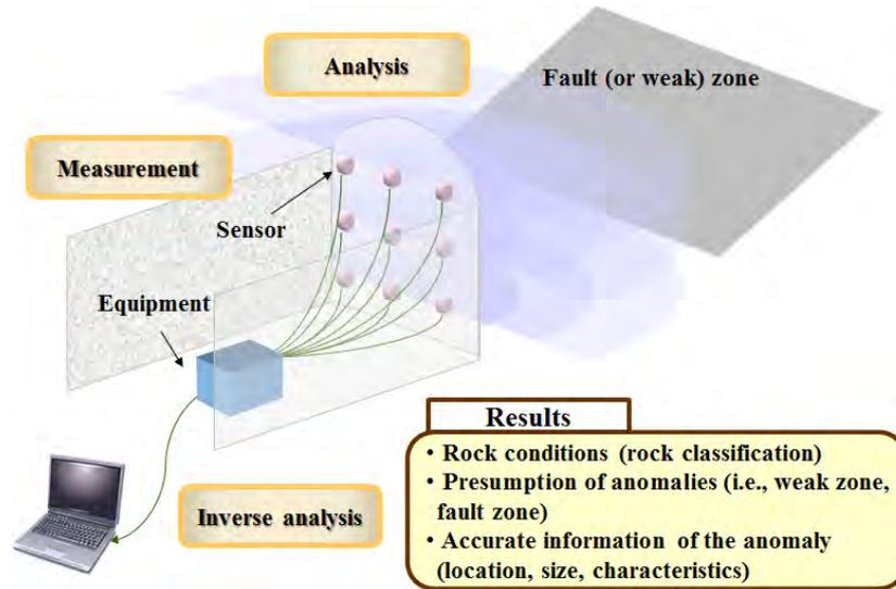
Fig. 1: Tunnel Electrical resistivity Prospecting System (TEPS).
