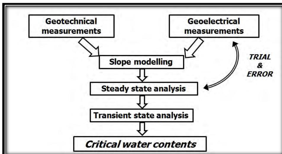
Fig. 1: Schematic diagram of the proposed geoelectrical-hydrogeological approach.
