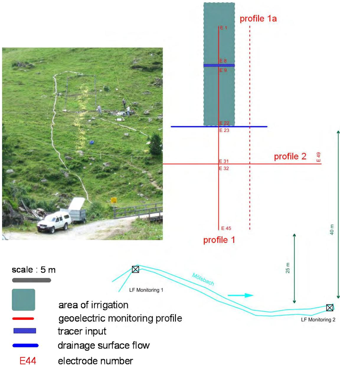
Fig. 2: Exemplified experimental layout (here: test site 1) for the assessment of shallow interflow velocities.
