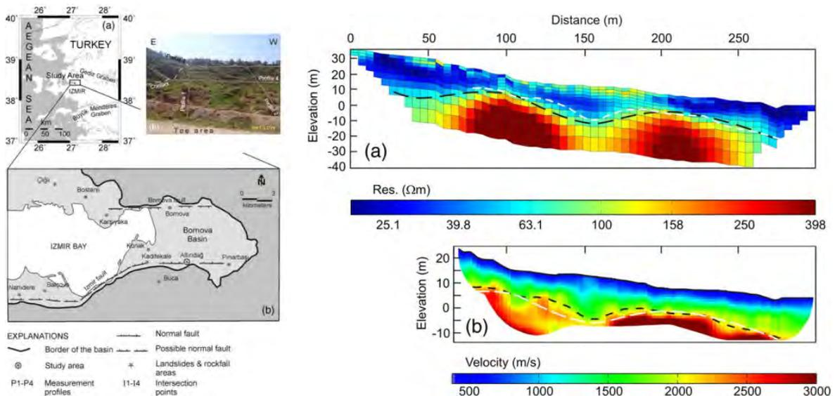
**Fig. 2:** Left: landslide area located in the Altındağ district of İzmir (Turkey). Right: (a) Resistivity tomogram together with the failure surface interpretations from the resistivity (black dashed line) and seismic data (white dashed line). (b) Velocity tomogram together with the failure surface interpretations from the resistivity (white dashed line) and seismic data (black dashed line) (modified from GÖKTÜRKLER et al., 2008).
