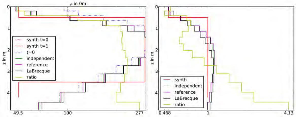
**Fig. 2:** Absolute resistivity (left) and relative changes (right) of different time-lapse strategies for a shallow infiltration front.
