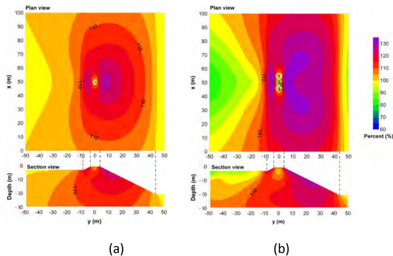
**Fig. 1:** Distortion of potential distribution by 3D effect caused by 3D dam structure when a homogeneous dam is excited by a pole (a) and dipole (b) source.
