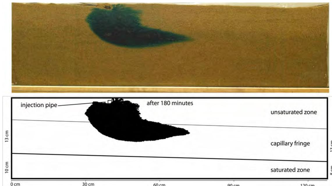
**Fig. 4:** Image analysis result from experiment 1 after 180 minutes, shown as photograph (upper) and outline of tracer plume from image analysis (lower).
