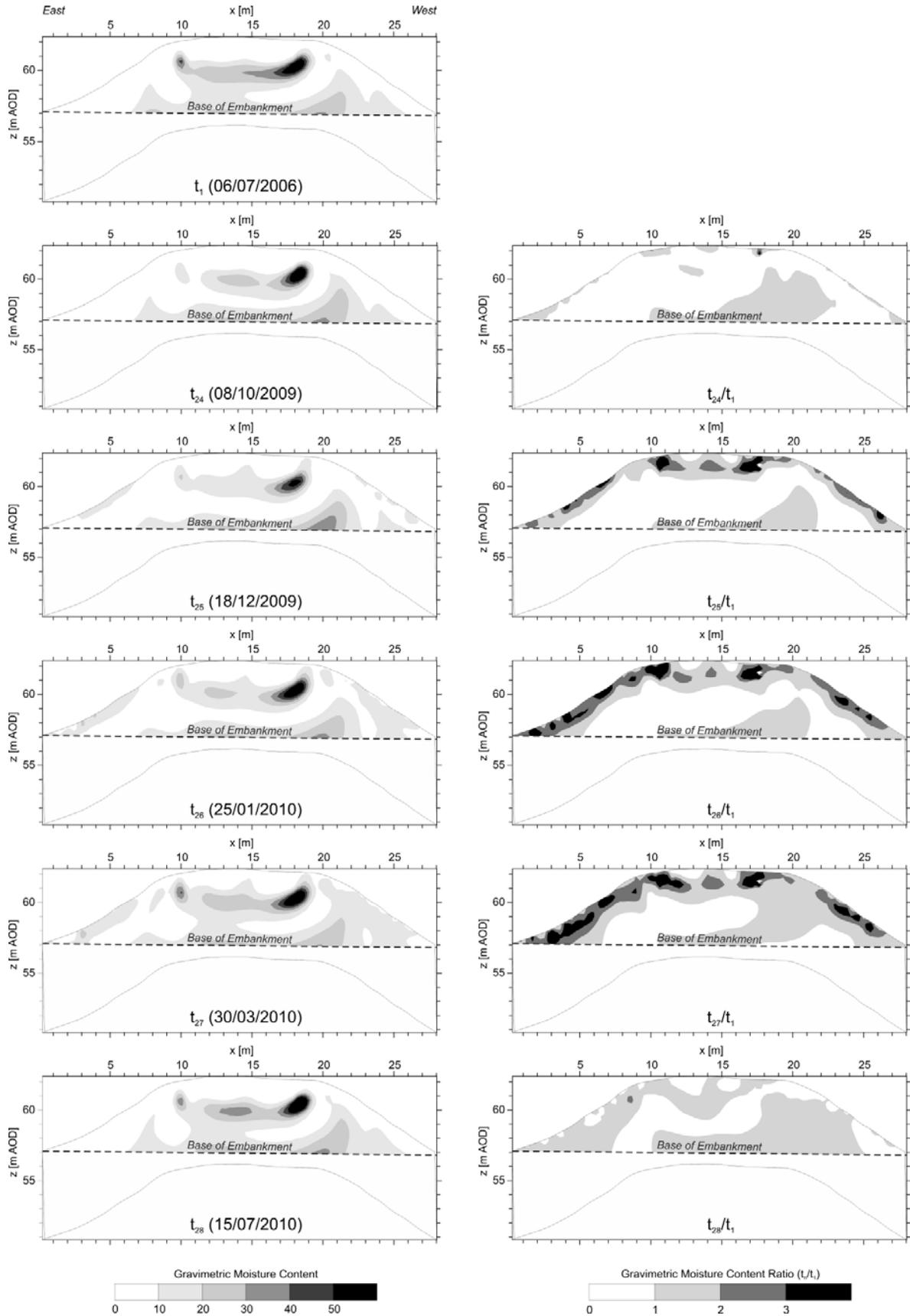
**Fig. 7:** ERT derived gravimetric moisture content (left) and ratio (right) plots calculated using the resistivity moisture content relationships determined from laboratory testing (Figure 5).
