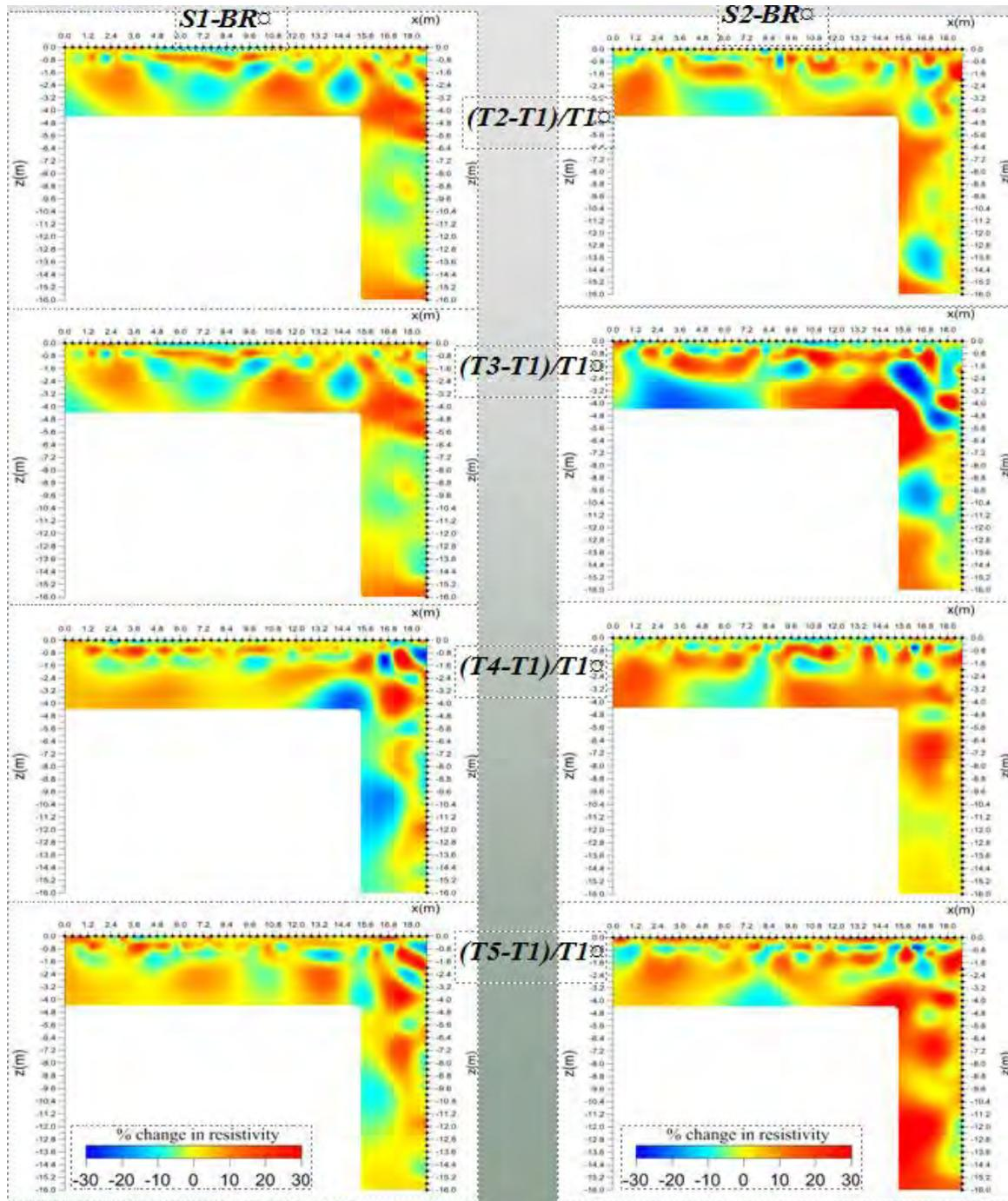
**Fig. 5:** Preliminary results of the difference inversion of the ERT data collected along lines S1-BRH and S2-BRH for the five time phases. The results are plotted in terms of percentage relative change of the model resistivity of each phase with respect to the reference phase.
