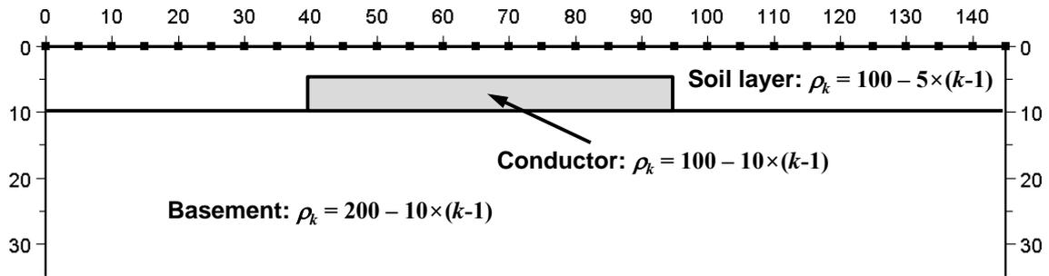
**Fig. 2:** A test model in which the resistivity throughout the entire modelled region is decreasing with time.  $\rho_k$  is the resistivity of each zone in  $\Omega\text{m}$  at the monitoring time step  $k$ .
