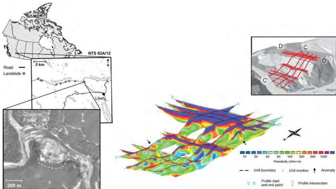
**Fig. 3:** Left: Landslide on the Quesnel River in British Columbia (Canada); right up: DTMs with DC electrical resistivity survey lines superimposed onto its surface; right bottom: 3D fence diagram of all resistivity data (modified from BICHLER et al., 2004)
