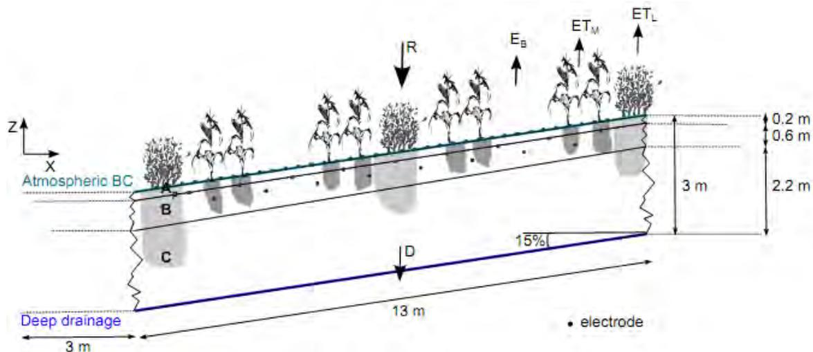
**Fig. 1:** Hydrological model set-up with top and bottom boundary conditions (BC) for a field plot with contour hedgerow intercropping with *Leucaena*, maize and bare soil strips. Three soil horizons are indicated on the scheme: Ap (0-0.2m), B (0.2-0.8m), C (0.8-3m). Symbols: ETM: evapotranspiration of maize rows, ETL: evapotranspiration of leucaena strips, EB: evaporation from bare soil strip, R: rainfall, D: drainage.
