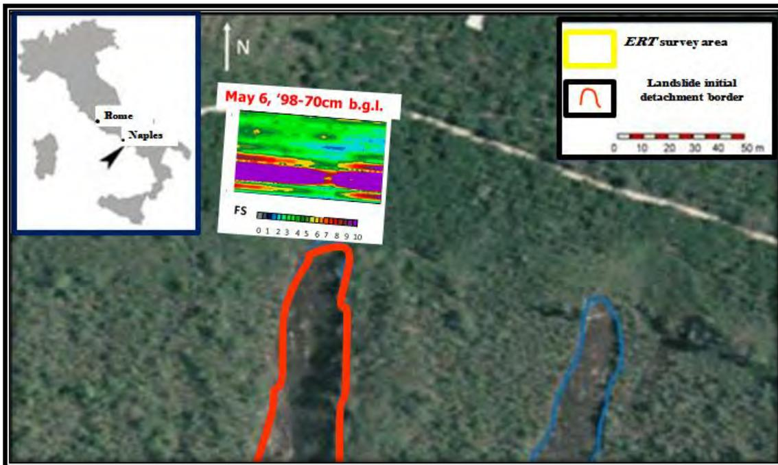
**Fig. 5:** Geophysical FS map of the survey area on May 5th, 1998, when the considered debris-flow event occurred. The FS values refer to a depth of 70 cm b.g.l. Note that the elongated strip characterized by FS values lower than surrounding is at the center of the initial detachment area marked with the red line.
