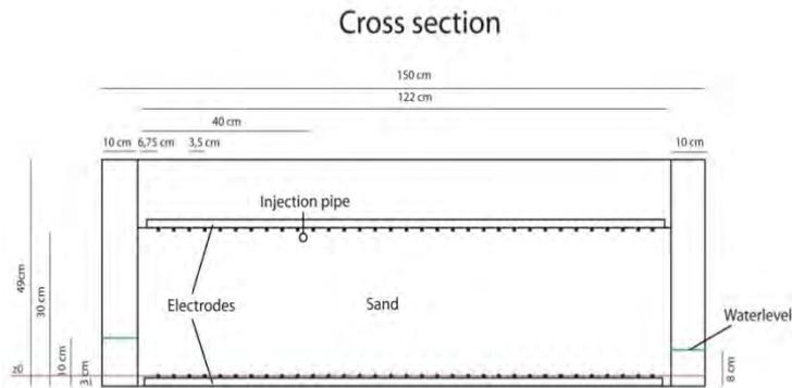
**Fig. 1:** Cross section of the aquarium layout.
