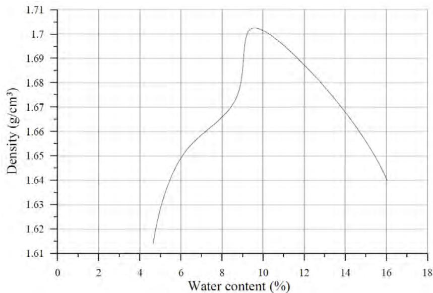
**Fig. 2:** Results of compaction test.
