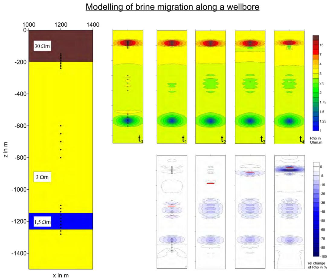
**Fig. 2:** Modelling of a brine upward migration in four steps. For modelling and inversion a bipole-bipole (cp-cp) configuration with an adapted geometry was used. The upper line shows the inversion results with  $t_0$  for the undisturbed model, the bottom line shows the differences ( $t_n-t_0$ ) of inverted results. The red line marks width and height of the saltwater column.
