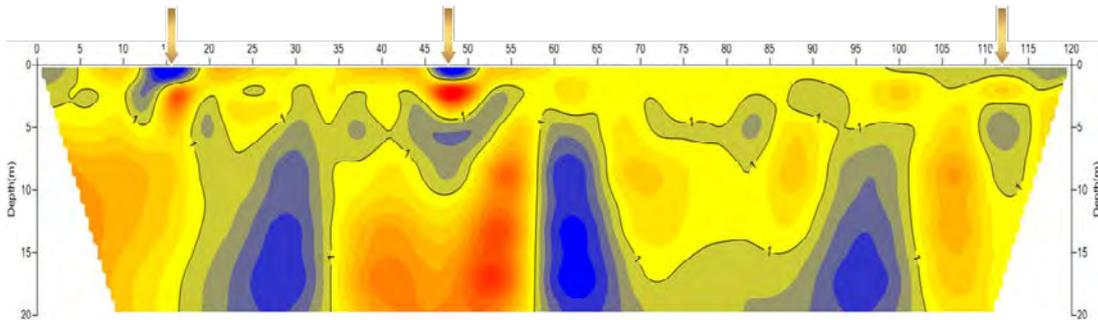
**Fig. 5:** The resistivity change ratio for Phase 10/Phase 1 on the dam crest after hydraulic fracturing.
