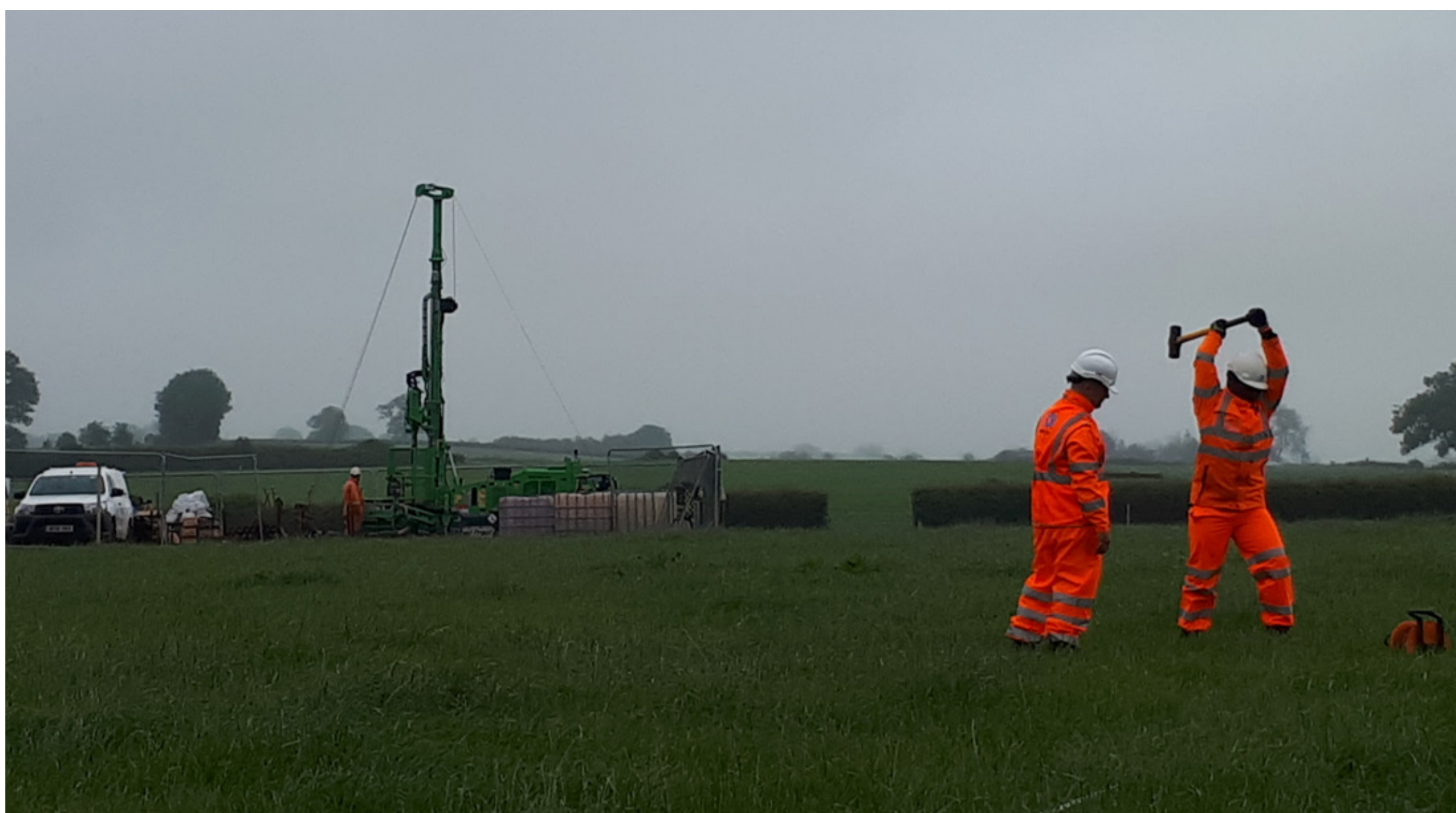
Figure 1: Image of data collection showing a seismic shot being undertaken using a hammer source.
