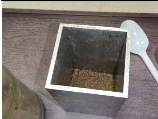
Formy do zagęszczania Molds for soil compaction
