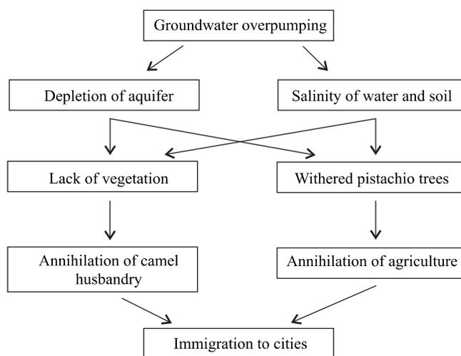
Fig. 1. Scheme of groundwater overexploitation impacts
