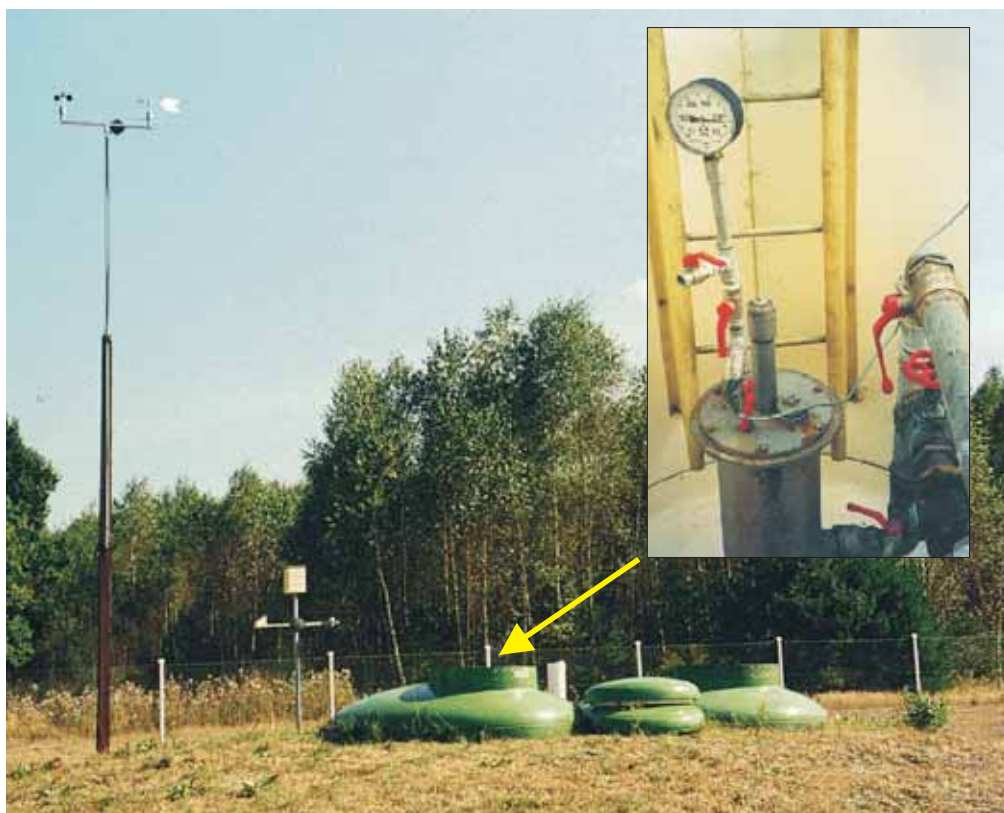
Fig. 1. Hydrogeological station of Polish Geological Institute — the observation network of groundwater body
