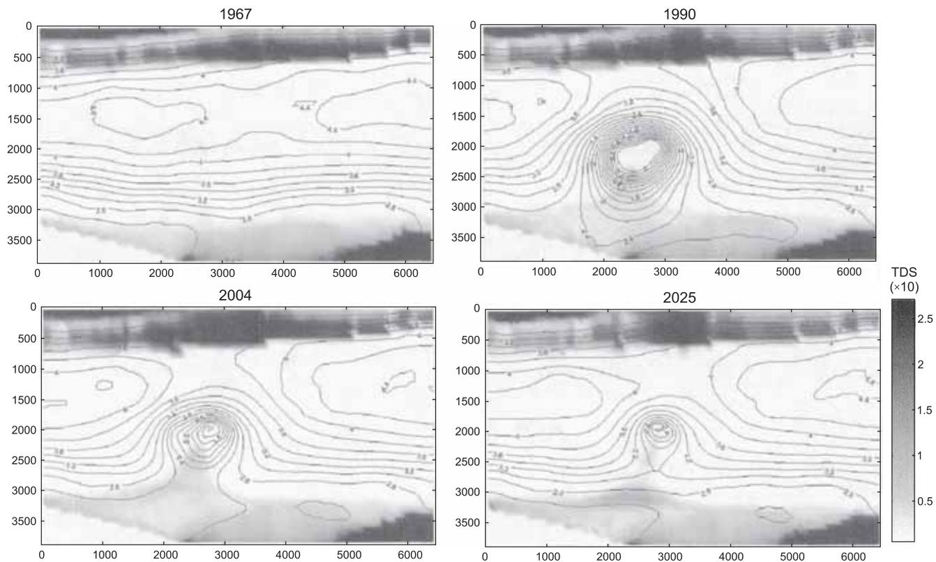
**Fig. 4. Horizontal cross-section along layer 8 for years 1967, 1990, 2004 and 2025 with indication of water quality distribution, hydraulic heads and groundwater flow**
