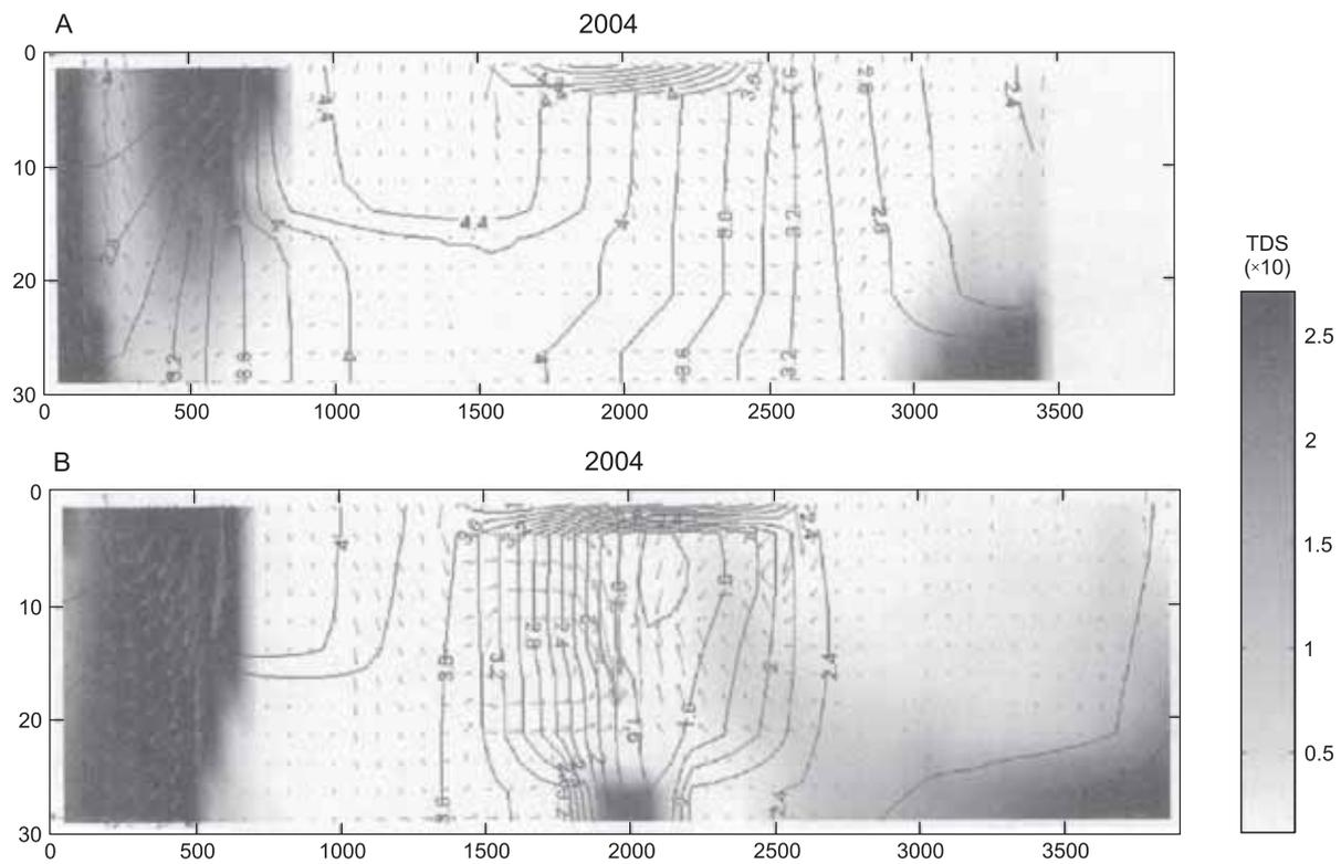
**Fig. 3. Vertical cross-sections along column 10 (A) and column 35 (B) with indication of water quality distribution, hydraulic heads and groundwater flow for the current situation**
