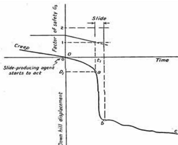
Fig. 1. Diagram showing factor of safety changes and slip surface movements preceding, during and after a landslide (after Terzaghi, 1950)
