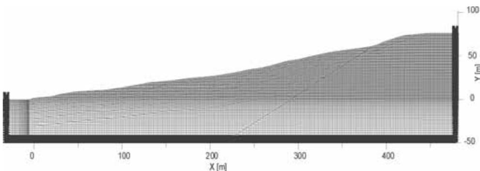
**Fig. 7. Kawiry landslide — finite difference grid**
