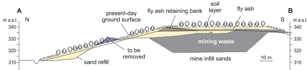
**Fig. 10. Cross-section of the area under recultivation**
