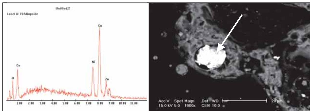
b) SEM image with EDS spectrum of aluminosilicate particles containing copper
