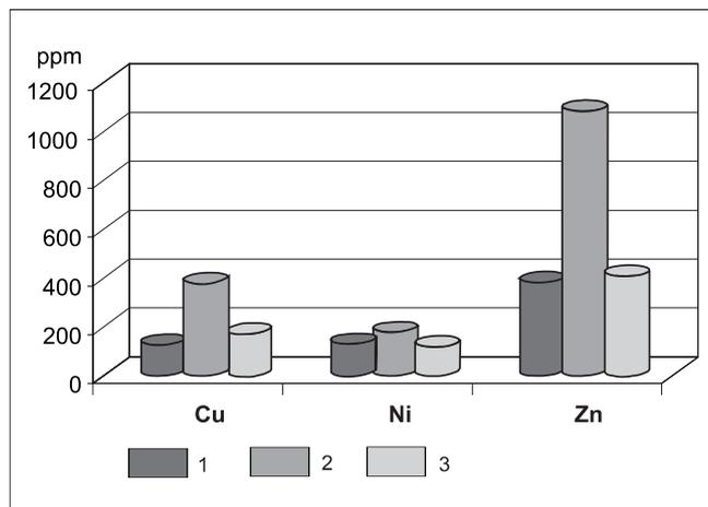
**Fig. 2. Average contents of Cu, Ni, and Zn (ppm) in the fly ash**
