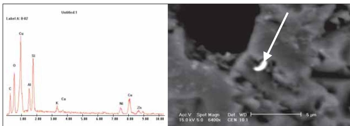
c) SEM image of zinc sulphide and "typical" EDS spectrum
