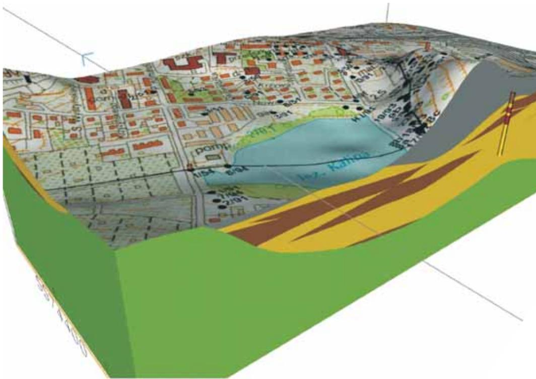
Fig. 4. Model geological cross-section (WE direction)
