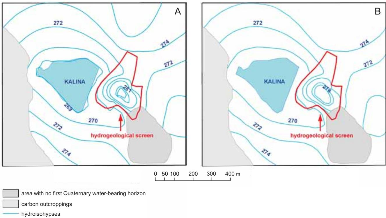
Fig. 5. A — Interpreted surface of water table of the first water-bearing layer;
