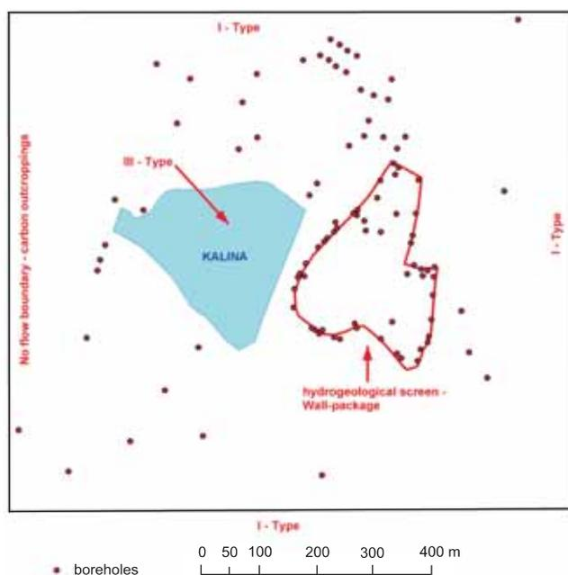
**Fig. 6. Boundary conditions for groundwater flow simulations**
