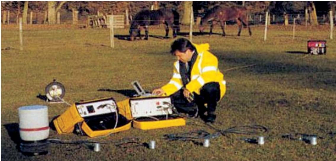
Fig. 7. Seismic velocity measurement
