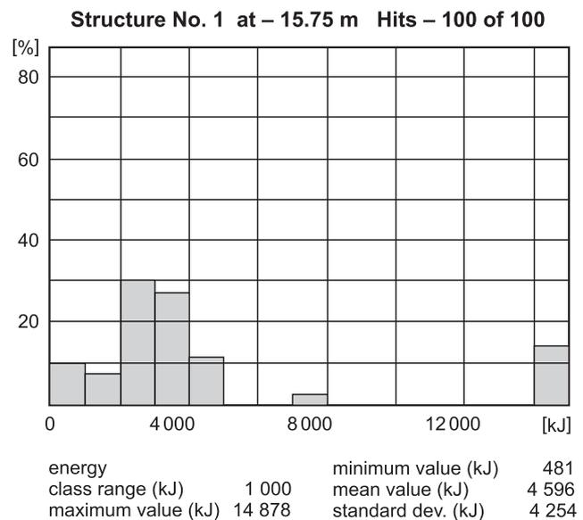
**Fig. 6. Expected energies along the catch fence**
