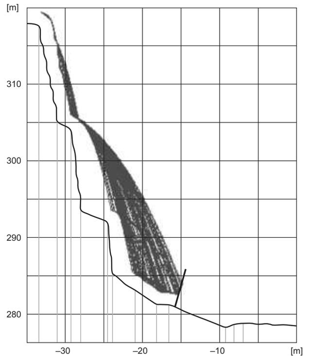
**Fig. 5. Trajectories of rockfall simulation**
