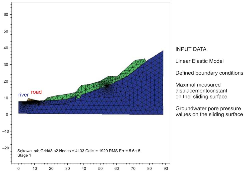
Fig. 6. Slope stability analysis FEM Method – final mesh
