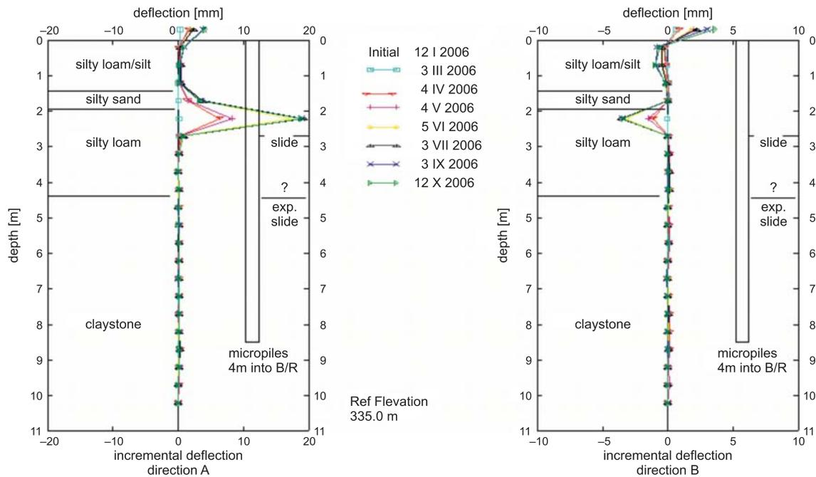
Fig. 2. Results of ground movement measurements
