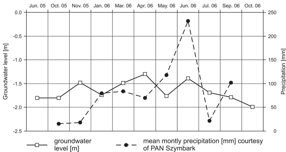
Fig. 5. Groundwater level and precipitation measurements
