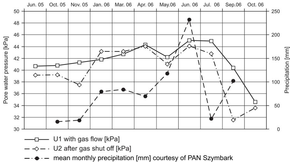
Fig. 4. Pore water pressures and precipitation monitoring
