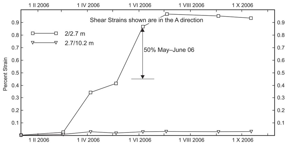
Fig. 3. Interpretation of mass movements measurements, displacement/shear strain plots
