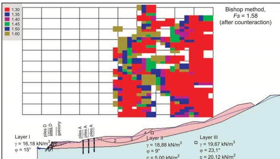
Fig. 8. Slope stability analysis with Bishop Method after proposed counteraction
