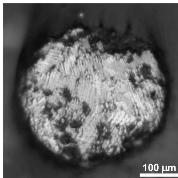
Fig. 4. Skeleton structure of magnetite and haematite particle (reflected light) from the fly ash from the heat and power stations in Upper Silesia (Poland)
