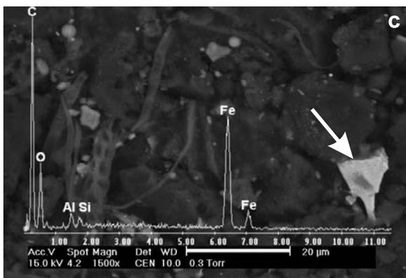
Fig. 1. Atmospheric particles of iron oxides from Chorzów (a), Katowice (b) and Sosnowiec (c)
