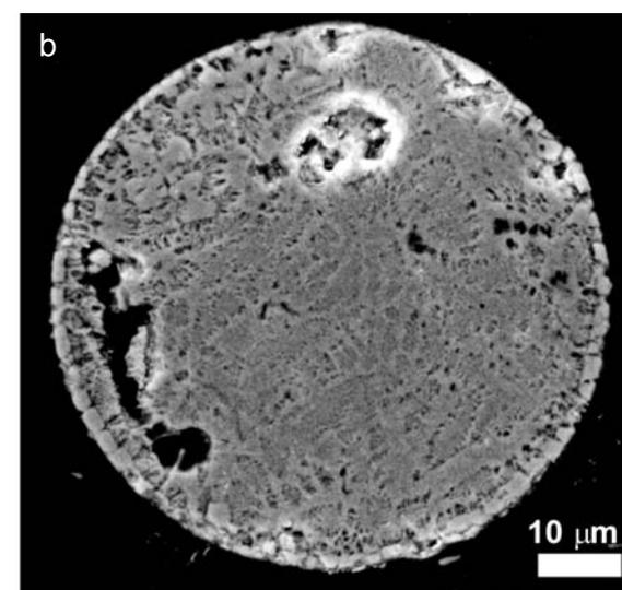
Fig. 5. Dendrite structure of fly ash particle (a) and atmospheric dust particulate (b)
