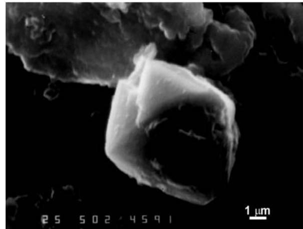
Fig. 2. Atmospheric particle of magnetite from Siemianowice Œskie, BSE image
