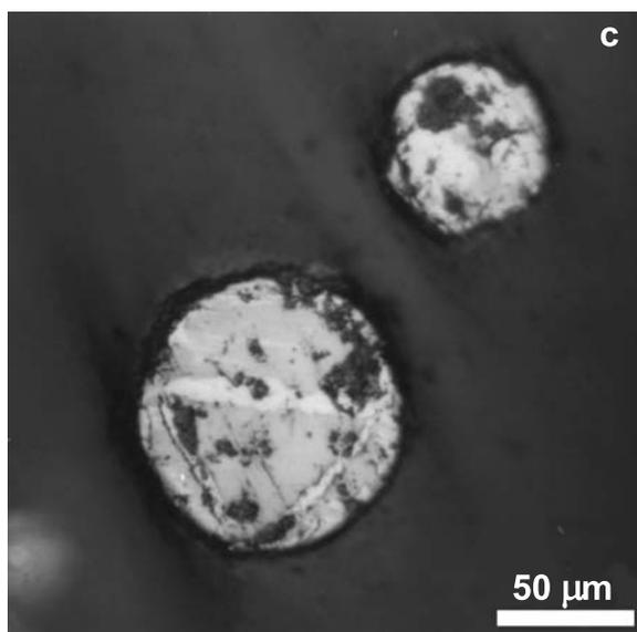
Fig. 3a, b — examples of iron oxides in the analysed fly ash in the heat and power stations in Upper Silesia (Poland) equipped with electrofilters; c — fan-shaped inclusions of magnetite and haematite in the aluminosilicate matter (reflected light); fly ash from the burning of bituminous coal in Upper Silesia (Poland)
